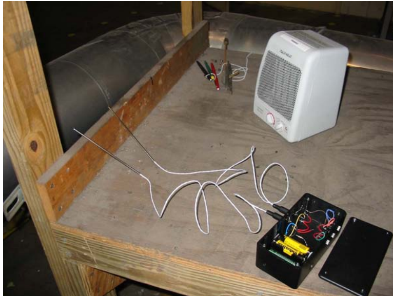
Figure 4-4 Heater and temperature probes at point “A”
