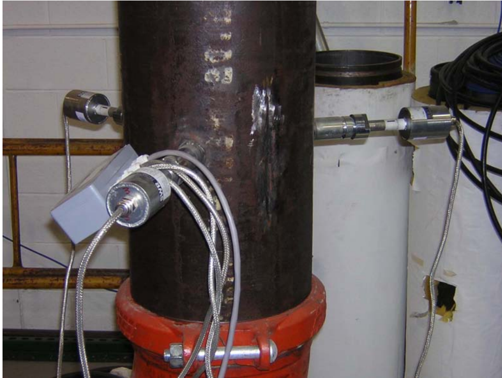
Figure 5-1 SolidFlow Sensors Installed in a Vertical Pipe Test Section of the Coal-Flow Loop
