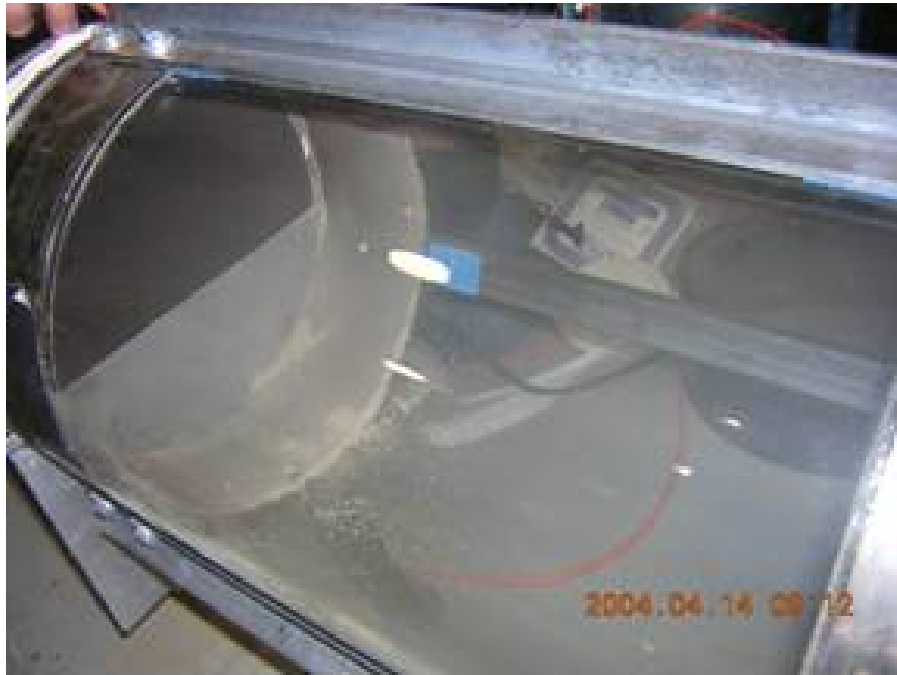
Figure 2-4 Segmental orifice located 12 diameters upstream of single 90-degree elbow
