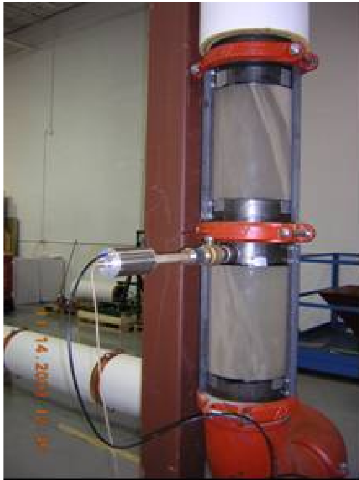
Figure 2-5 Photo of roping flow with ceramic particulate at Location 3V3
