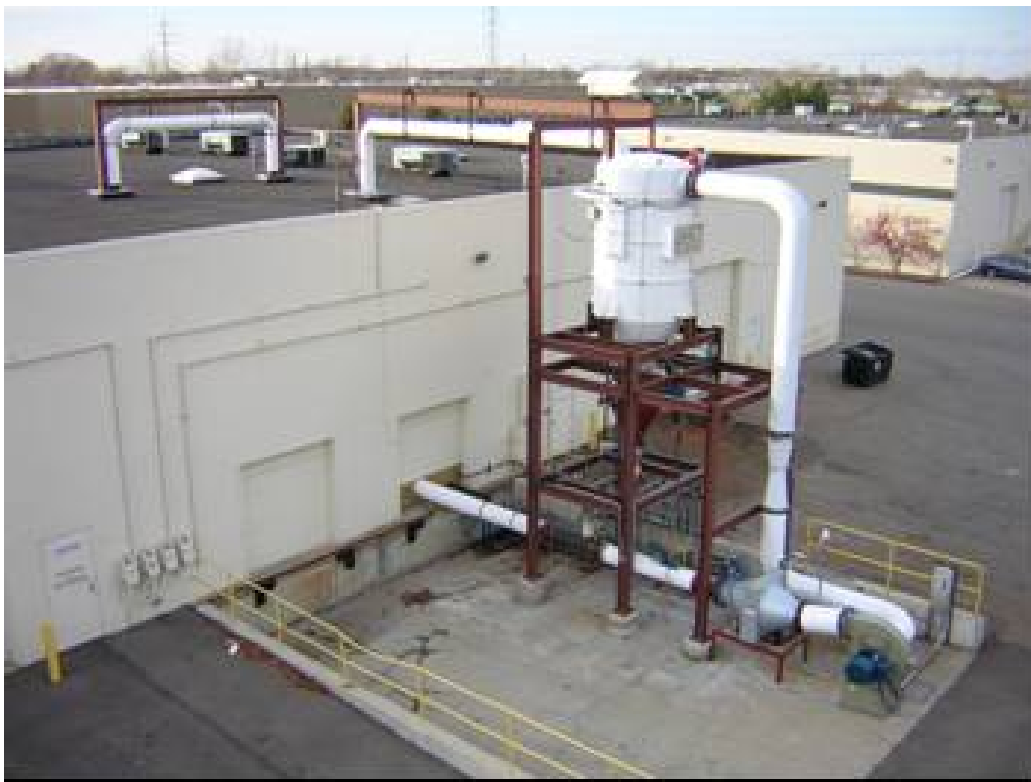
Figure 2-1 EPRI's CFL facility was expressly designed to measure the mass flow rate of pneumatically transported pulverized coal. This exterior photo shows the filter/receiver, storage hopper, and cleaned carrier gas outlet.
