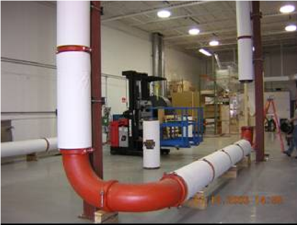
Figure 2-2 The coal loop closely replicates the scale and flow conditions of a typical coal plant.
