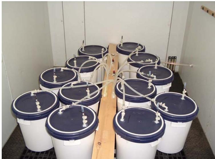
Figure 2-3 Air sampling of multiple containers of concrete in the environmental chamber
