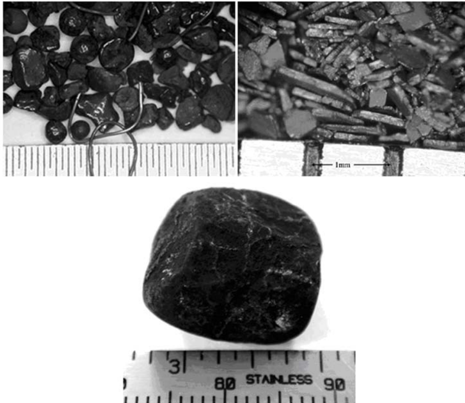
Figure 7-2 Examples of Debris Found in HRSG Tubing (Shot Blast Media, Exfoliated Oxide Scale, and a Rock-Like Particle)
