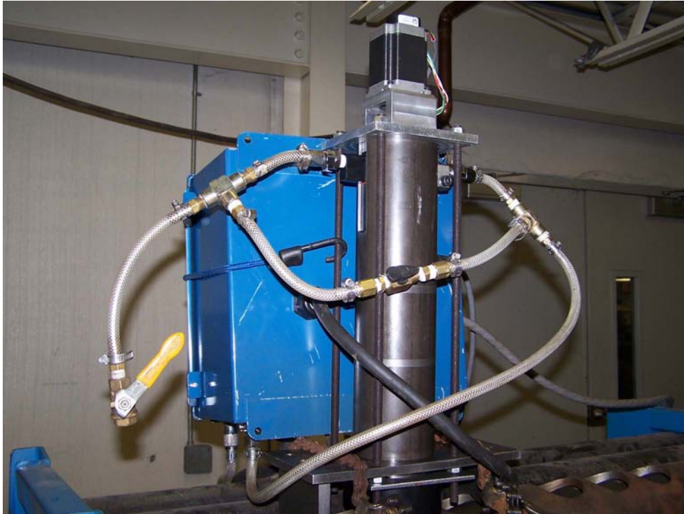
Figure 3-6 A Contoured EDM Profile Device is Used to Remove the Damaged Header-to-Existing Weld
