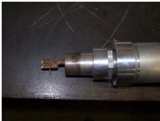
Figure 3-28 A closer view of ID Tube Welding Head shown in Figure 3-27
