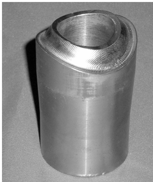
Figure 3-22 Upper Profile of Tube Fabricated to Match Contour of Header ID
