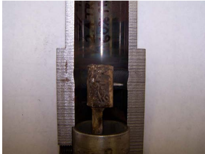
Figure 3-29 The ID Tube Weld Head Is Shown Inserted Into a Cut-away of a Tube (top) to Stub Tube (bottom) Mockup. Tube Diameter is 1-1/4 inches.
