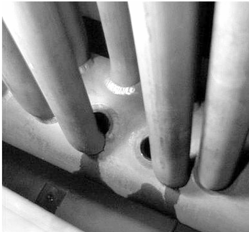
Figure 3-1 Failed HRSG Tube at the Header Location
