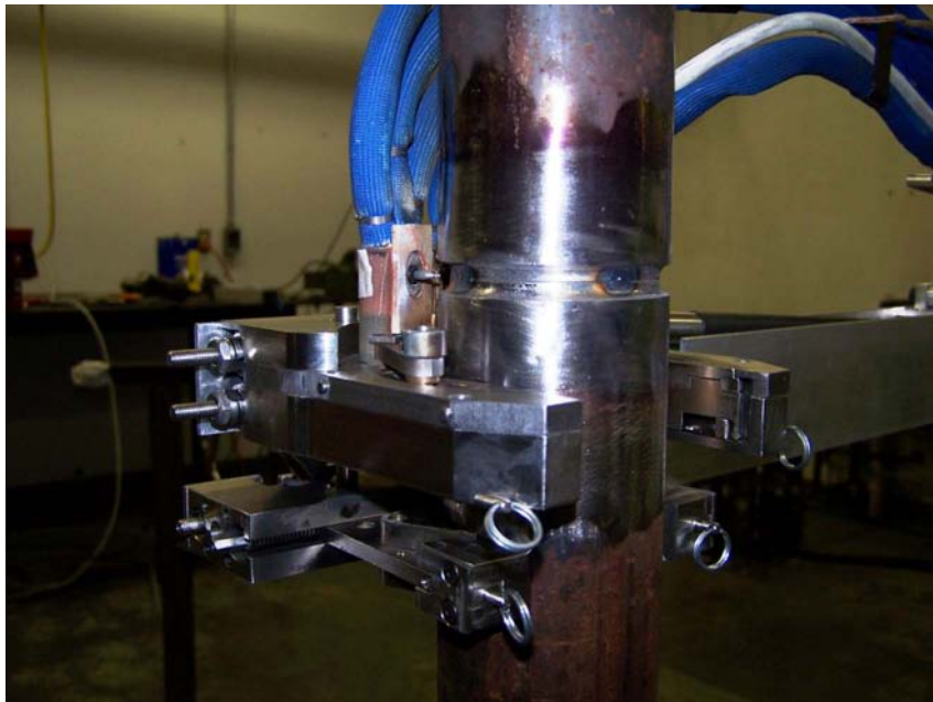
Figure 3-19 Another view of the C-Frame welding approach used for CANDU reactor tubing.
