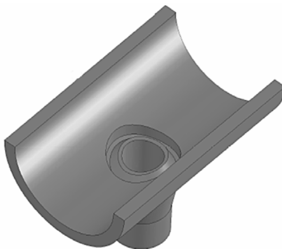
Figure 3-30 Schematic Showing ID of Header with Stub Tube Inserted
