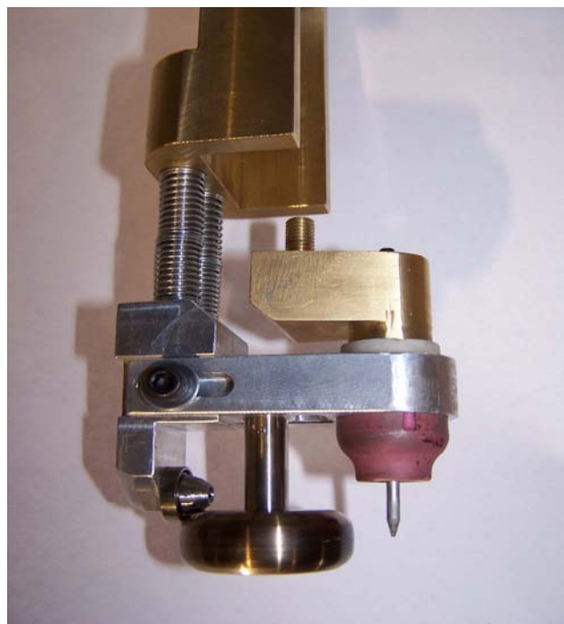
Figure 3-33 A cam follower is an integral part of the ID header welding device.
