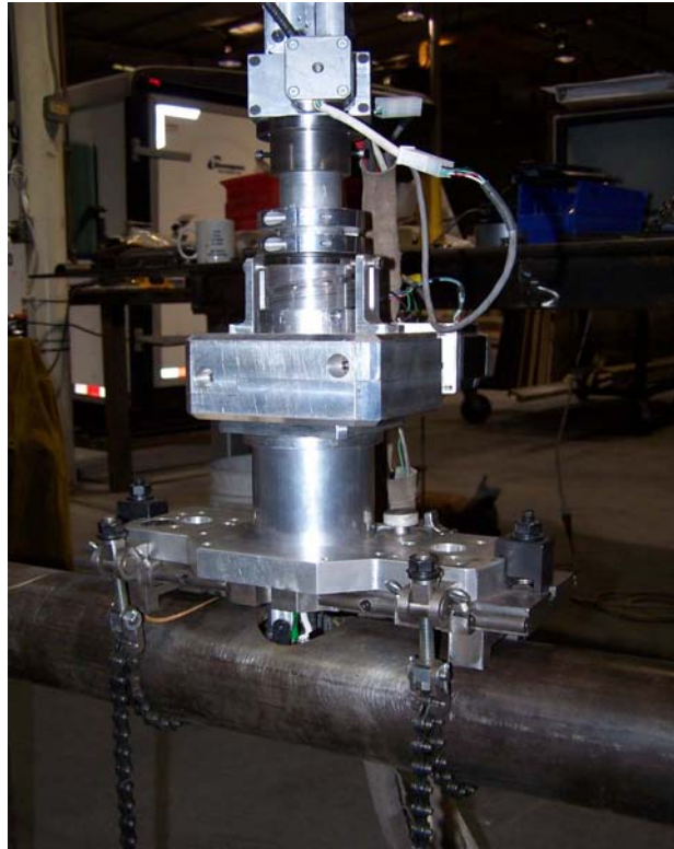
Figure 3-32 Header-to-stub tube welding device inserted into a header.
