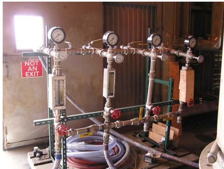
Figure 4.3. Flow control system
