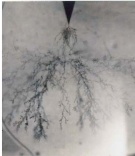
Figure 5-4 Examples of Electrical Trees in XLPE Insulation [15]
