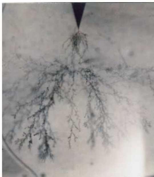
Figure 5-4 Examples of Electrical Trees in XLPE Insulation [15]
