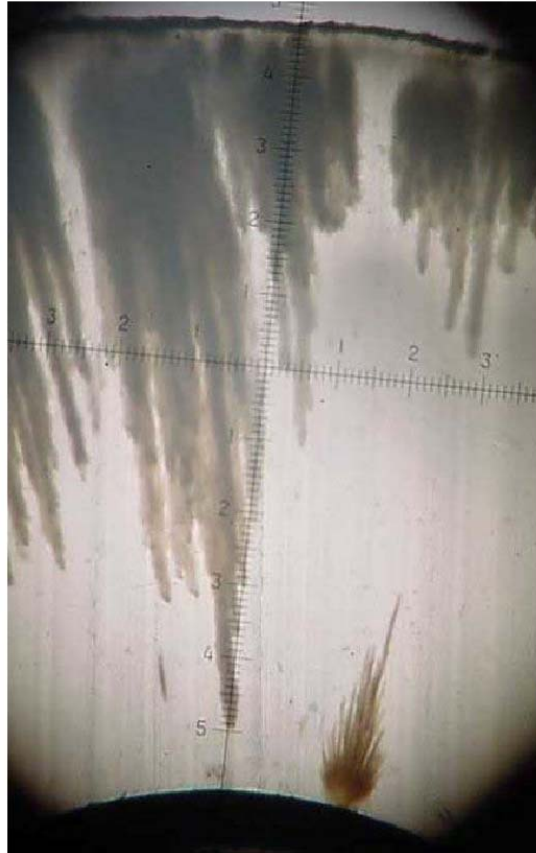
Figure 5-2 Example of Vented Trees Growing from Conductor and Insulation Shield Interfaces [15]
