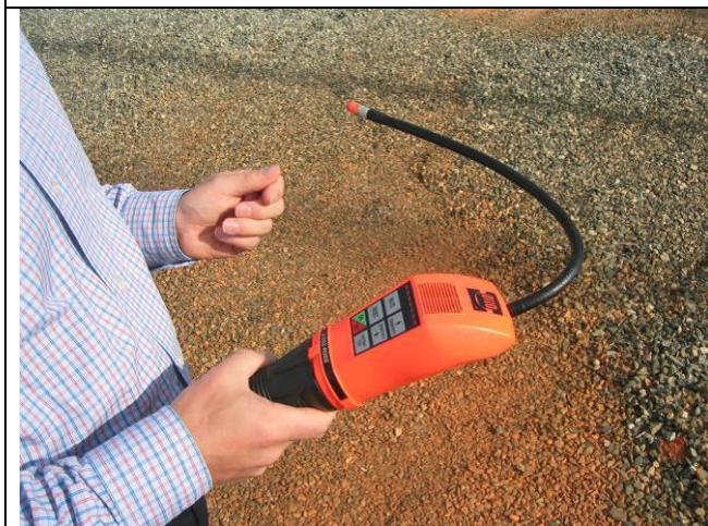
Step 5: Final leak detection to prove the seal
