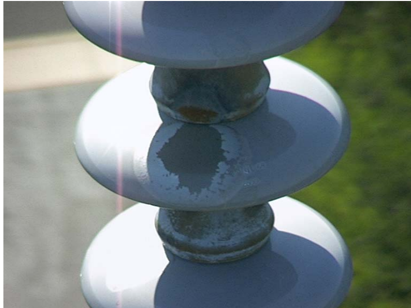
Figure 1-6 Example of an Insulator String that Flashed Over
