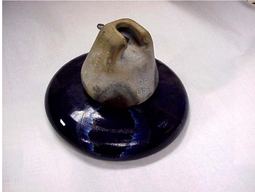
Figure 1-5 Example of an Insulator that Flashed Over
