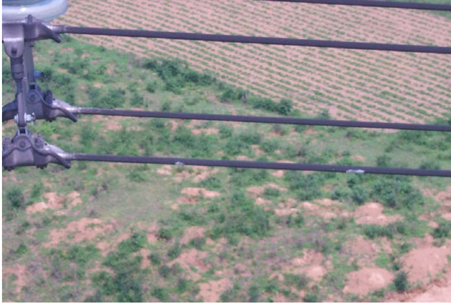
Figure A-10 Evidence of a Sparkover (Burn Mark) on Conductor Hardware
