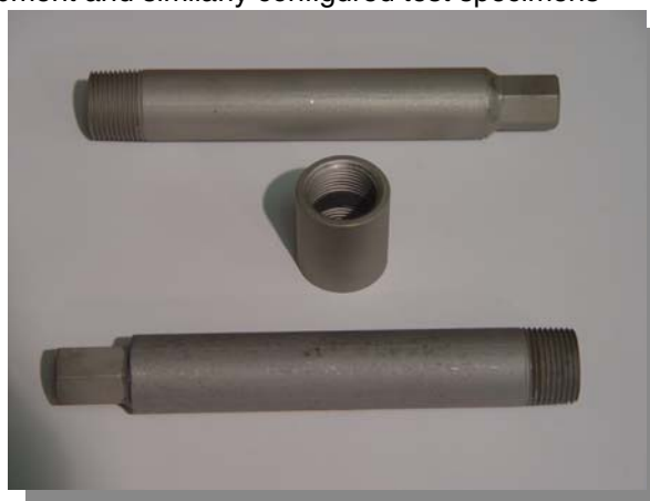
Figure 1 Test Specimen Piping Components
