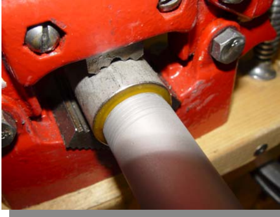
Figure 4 Correct Seal Bead Formation Post-
