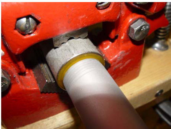
Figure 4 Correct Seal Bead Formation Post-
