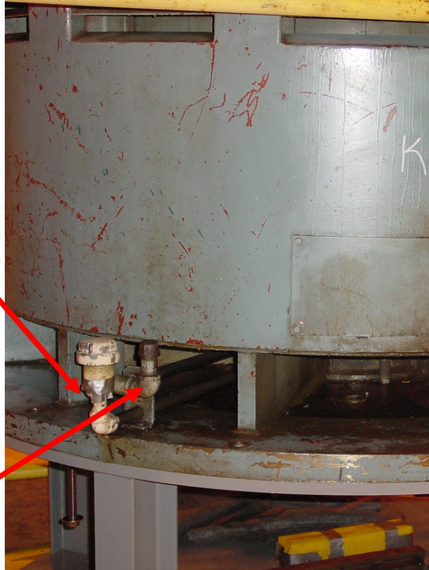
Figure 4-29 Lower Bearing Potential Leak Paths
