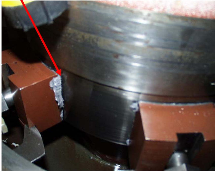
Figure 4-20 Lower Bearing Oil Damage from low oil level
