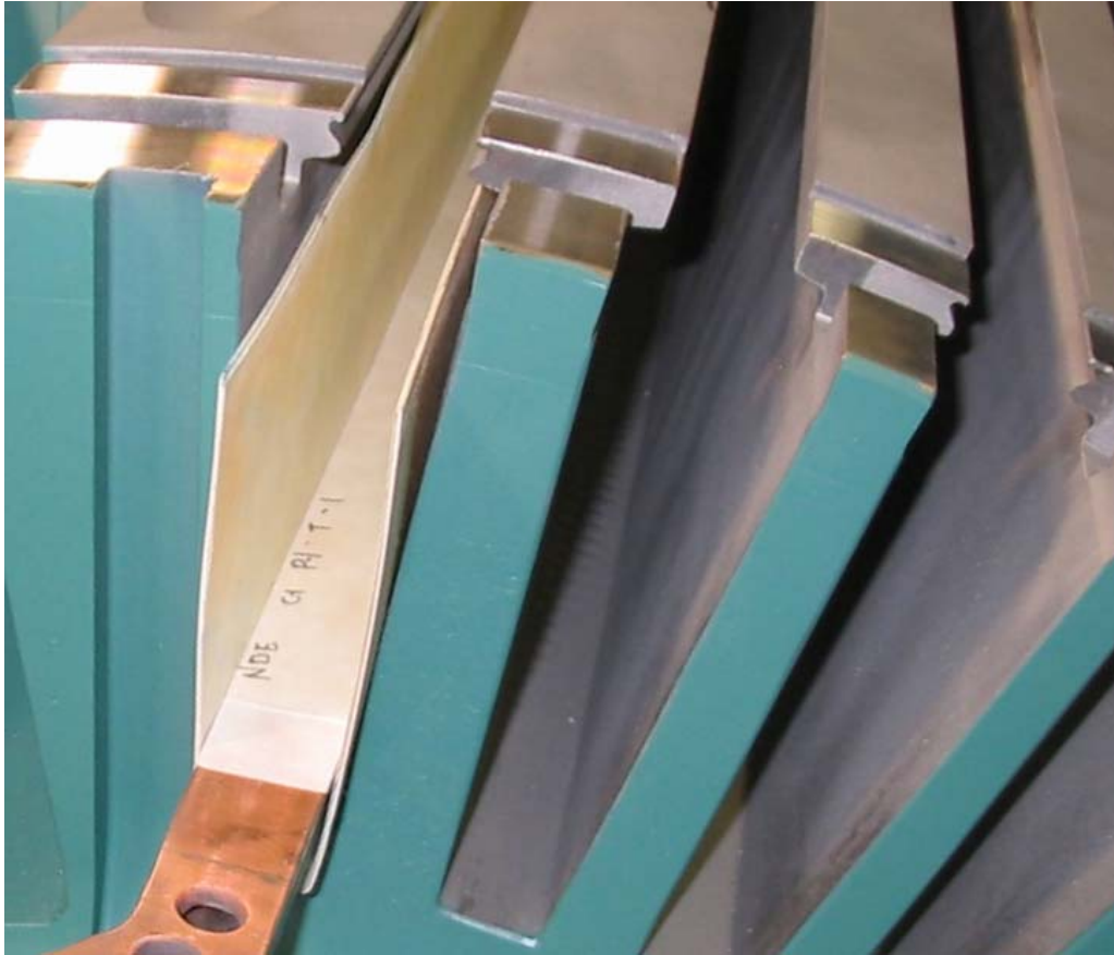
Figure 2-11 Turn Insulation and Ground Wall Insulation with One Turn Installed
