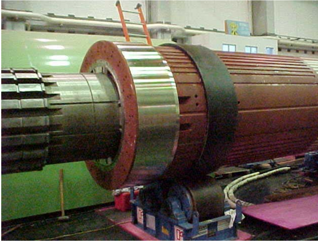
Figure 4-4 Rotor with Retaining Ring and Centering Ring
