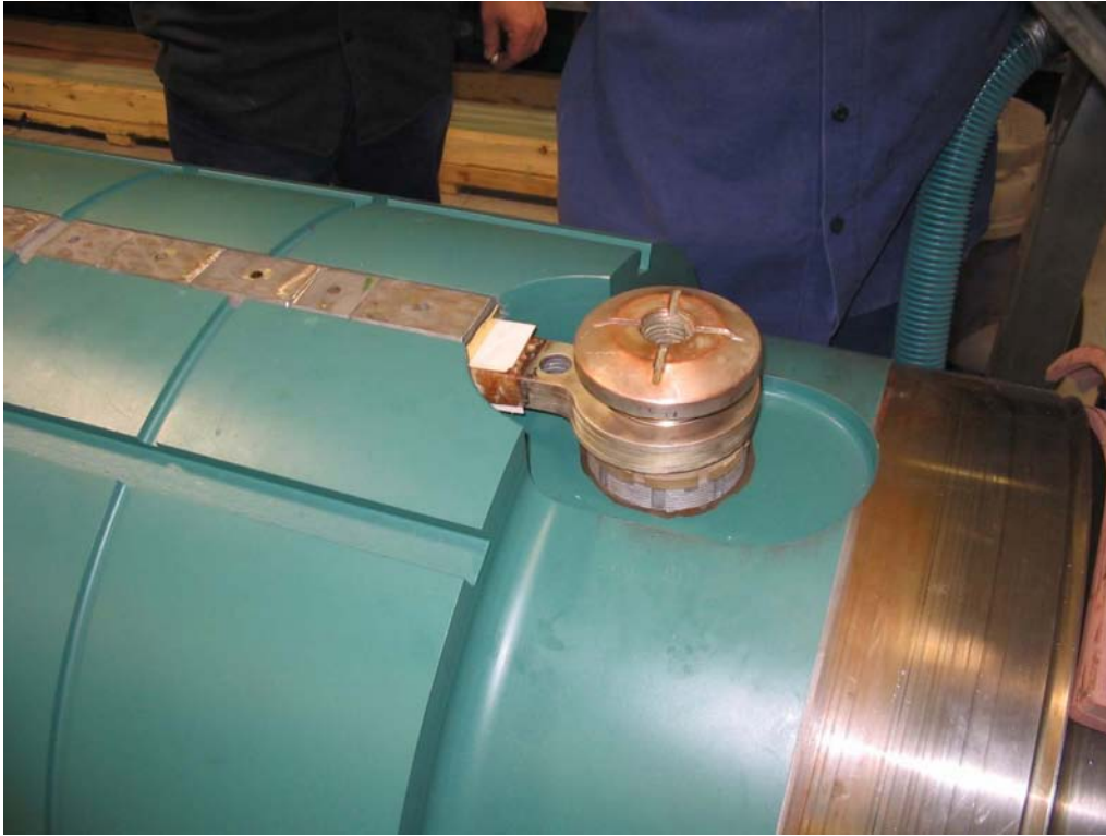
Figure 4-6 Radial Stud with Field Lead
