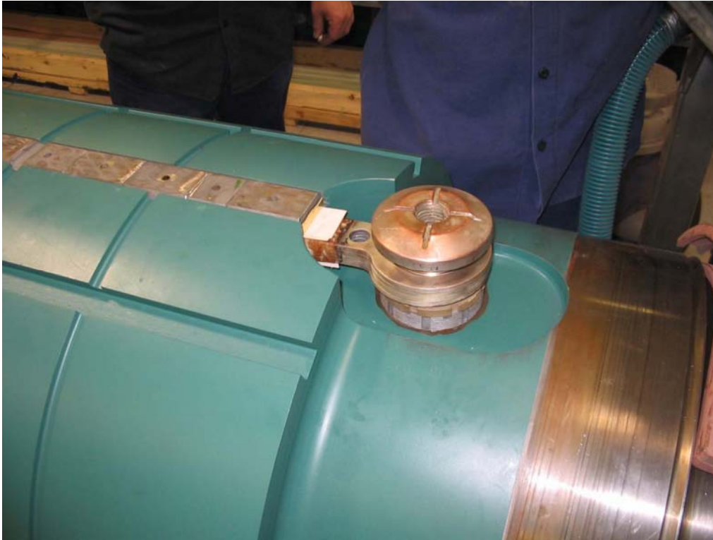
Figure 4-6 Radial Stud with Field Lead
