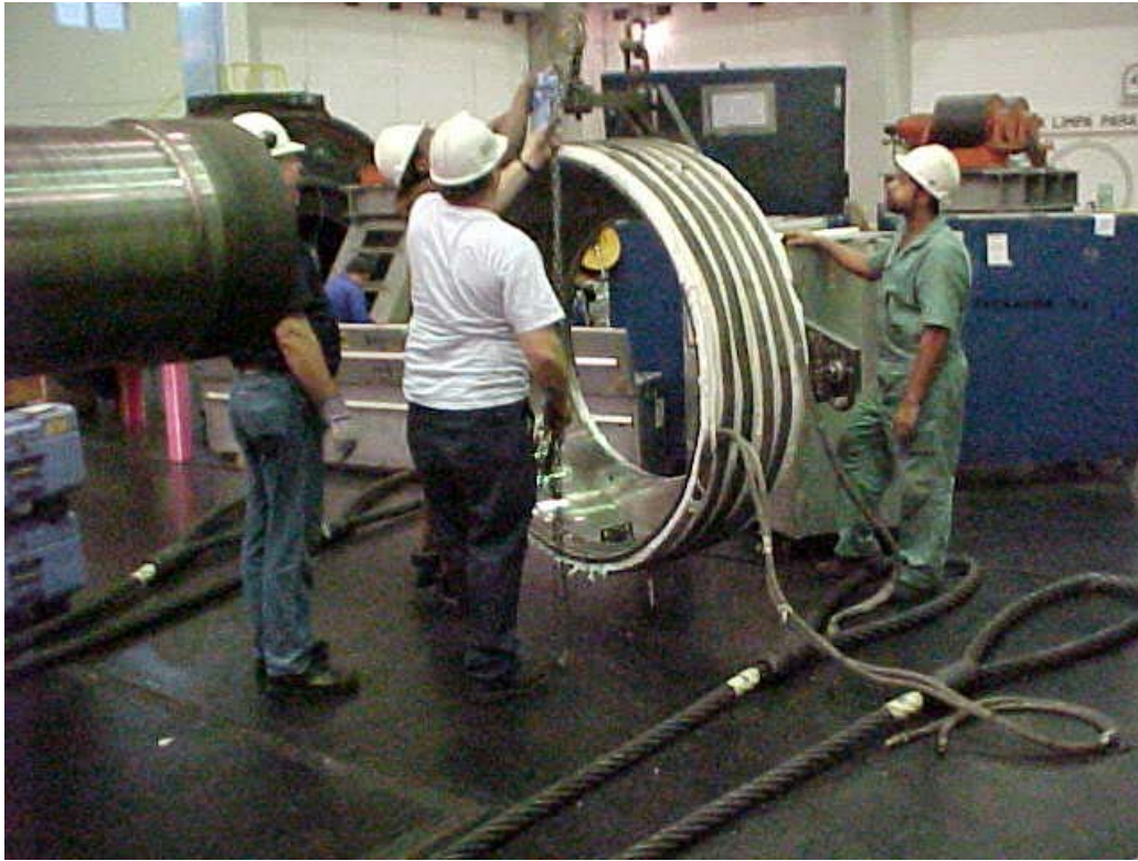
Figure 2-9 Retaining Ring Removal, Note Heating Coil
