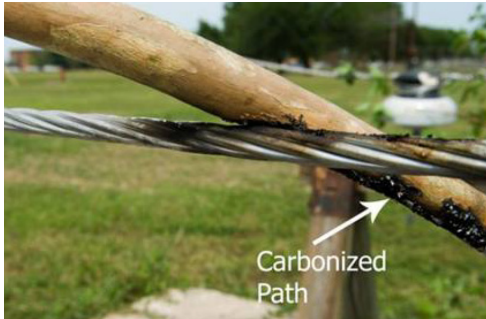
Figure 4-2 Carbonization, or “Char,” Created When Vegetation Bridges Conductors
