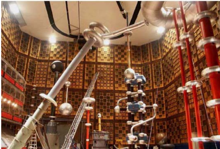
Figure 8-2 800 kV DC Bushing (Courtesy of Siemens)
