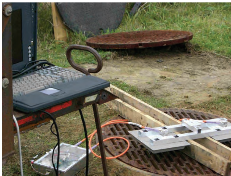
Figure 1-6 Reader with Antennas Positioned Above the Slotted Steel Manhole Cover
