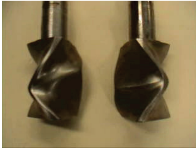
Figure 2-4 Roller Type High Shear Rotors Used by Both RPI and Dow
