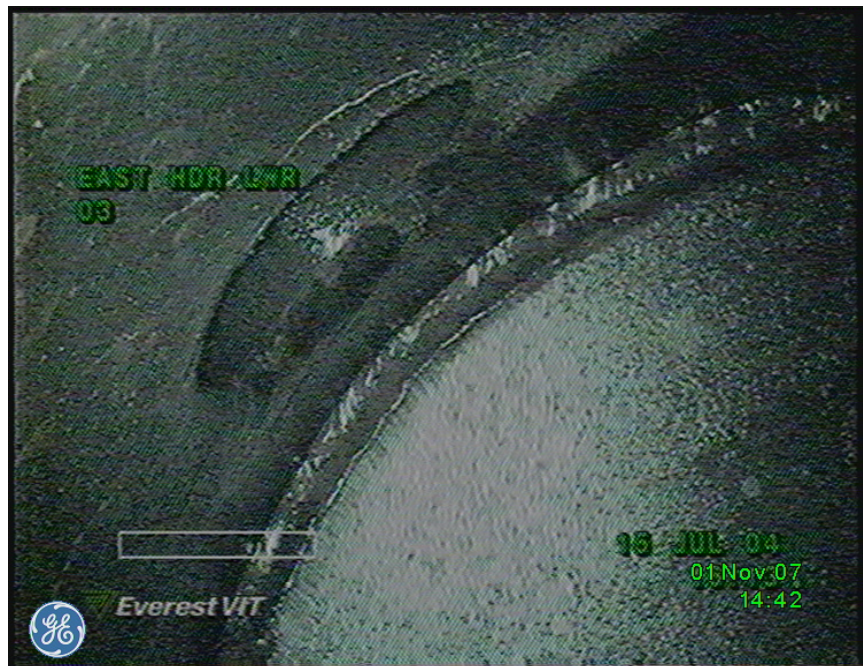
Figure 7-2 Additional RVI Image of the Upper Economizer with Significant Surface Deposit (Deposit is more than what would be expected from normal properly treated service.)
