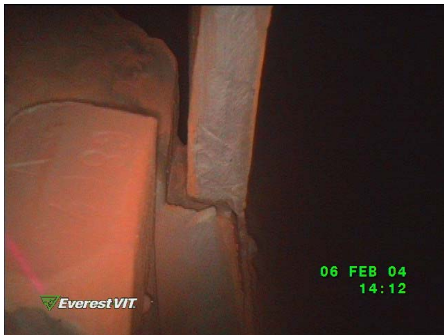
Figure 4-3 RVI Image of Cracking in an Attenuator Nozzle (Cracking may progress and lead to failure of the nozzle.)
