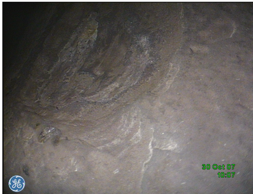
Figure 6-2 Layered Deposit on a Pitted Area in a Waterwall Tube as Seen in Figure 6-1
