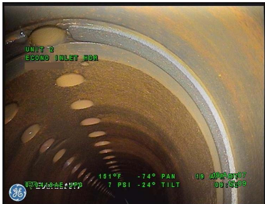
Figure 3-9 Clean Header Condition Can Be Documented with RVI
