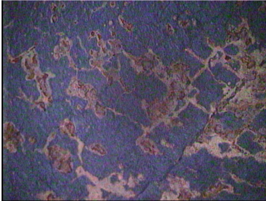
Figure 5-7 More Severe Crazed Cracking Than That Seen in Figure 5-3 (Some of the oxide layer has spalled in this region.)
