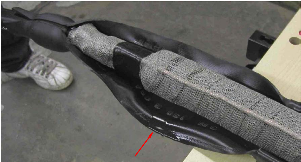
Figure C-6 Joint 3M7. Water Accumulated Under the Jacket of the Joint.
