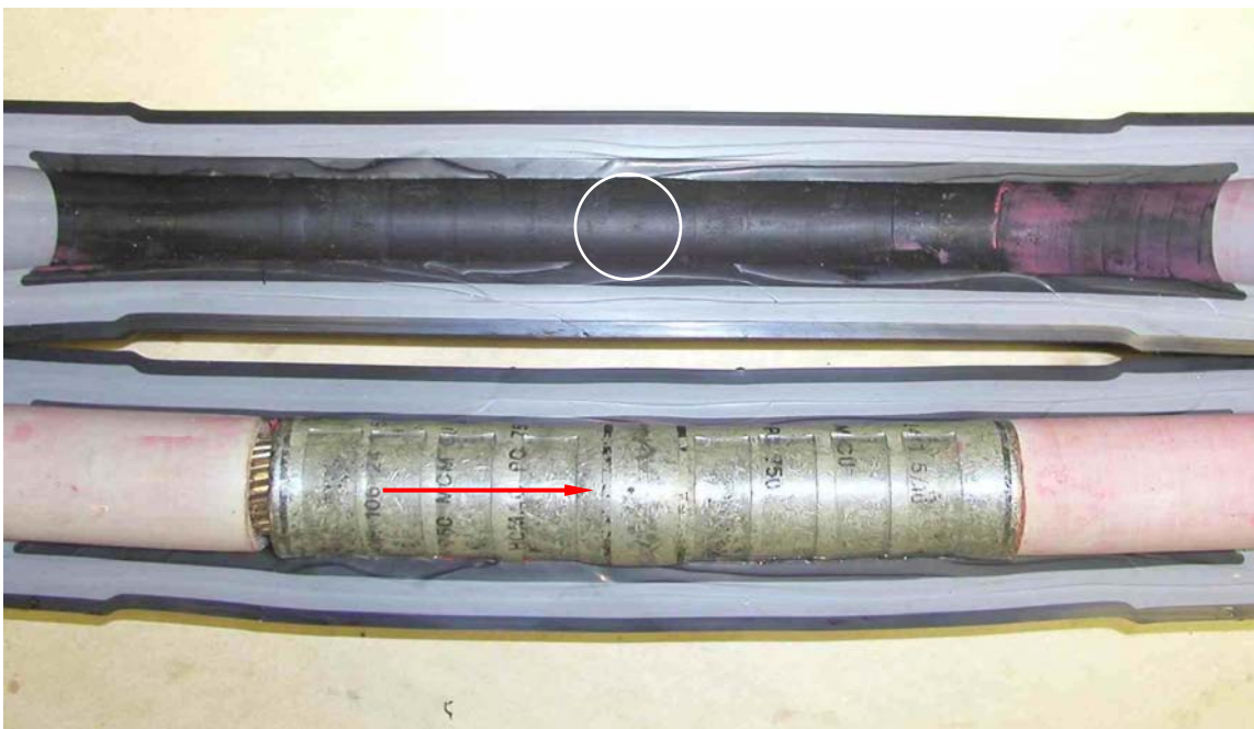
Figure C-3 Joint 3M4. Radial Failure at Center of the Connector.
