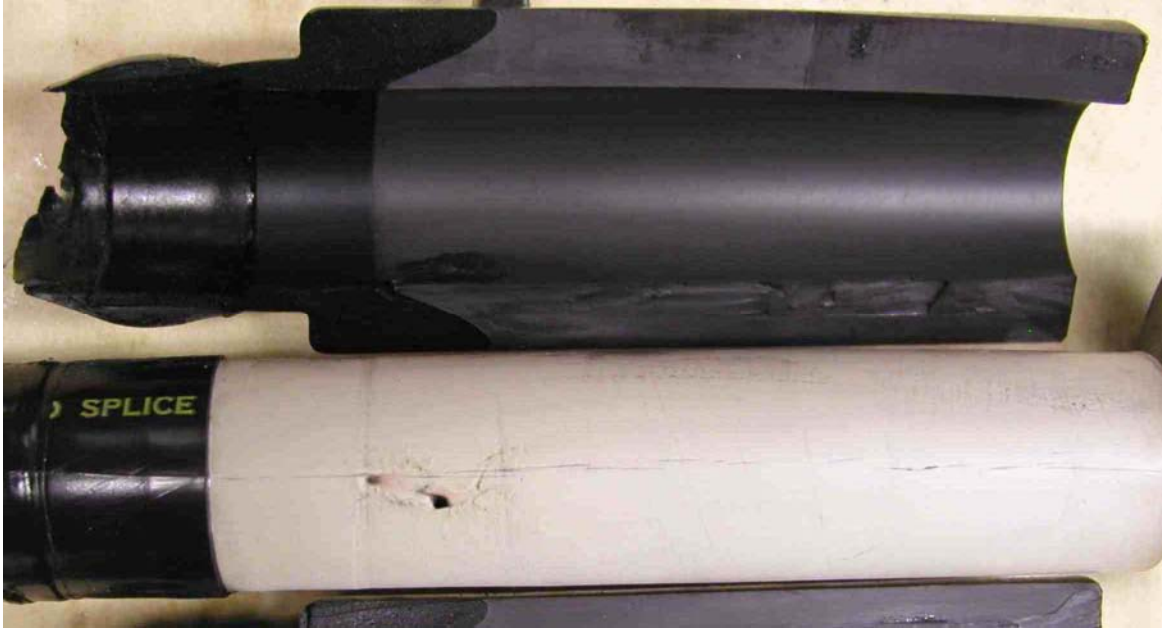
Figure D-3 Joint E8 (with Retaining Ring). Radial Failure at About 0.4 Inch from Semiconducting Layer of Cable Adapter.
