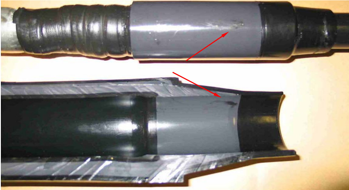
Figure E-3 Joint R2. Longitudinal Failure at the Interface Between the Insulation of the Cable Adapter and Receptacle Housing.
