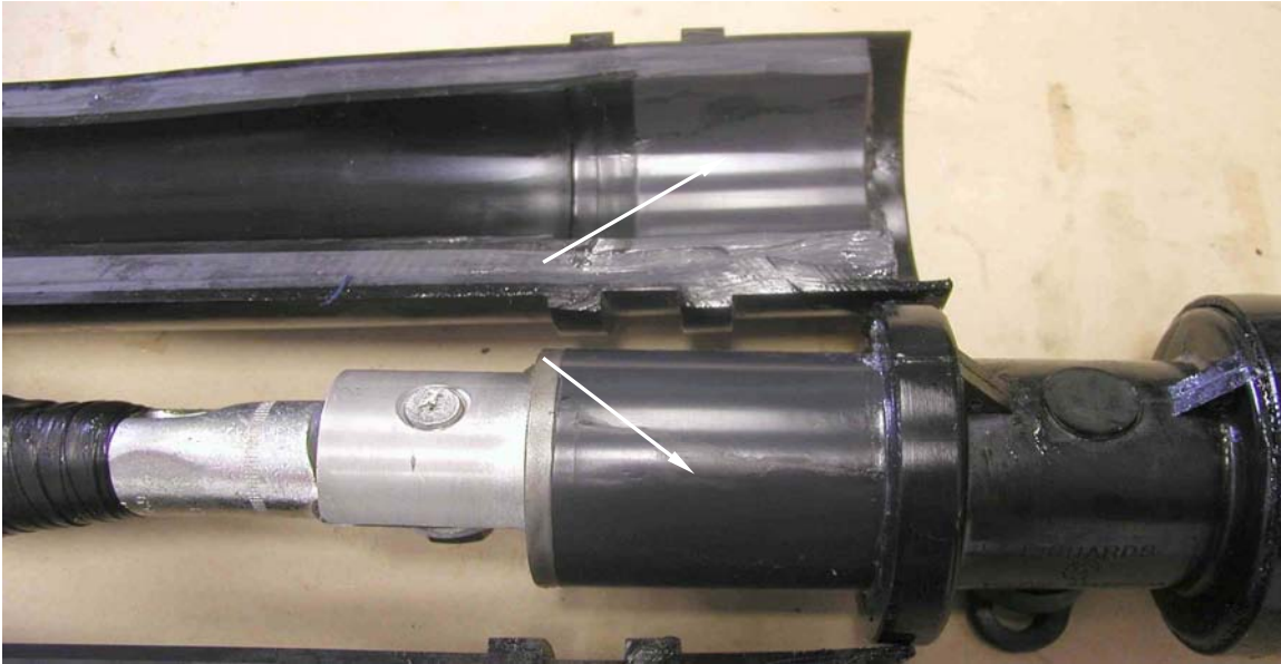
Figure F-1 Joint R4. Longitudinal Failure at the Interface Between the Insulation of the Bus Bar and Receptacle Housing.
