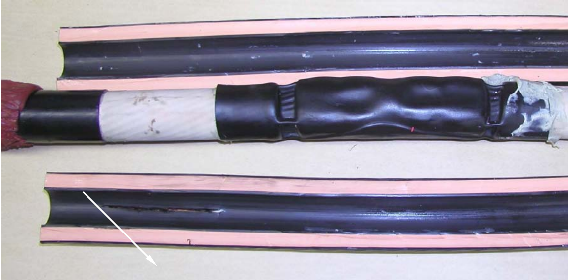
Figure A-1 Longitudinal Failure in Joint T7.
