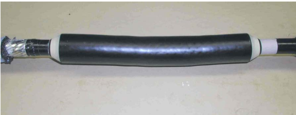
Figure B-4 Joint P6. Joint Body Not Properly Centered
