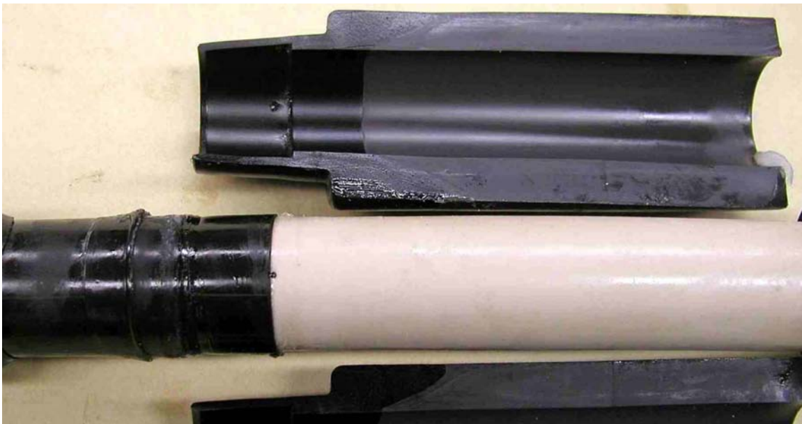
Figure D-4 Joint E6 (with EPR Tape Bumper). Radial Failure at the Cable Insulation Shield Cut Back.
