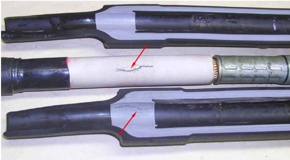
Figure C-1 Joint 3M1. Longitudinal Failure at the Interface Between Joint and Cable.
