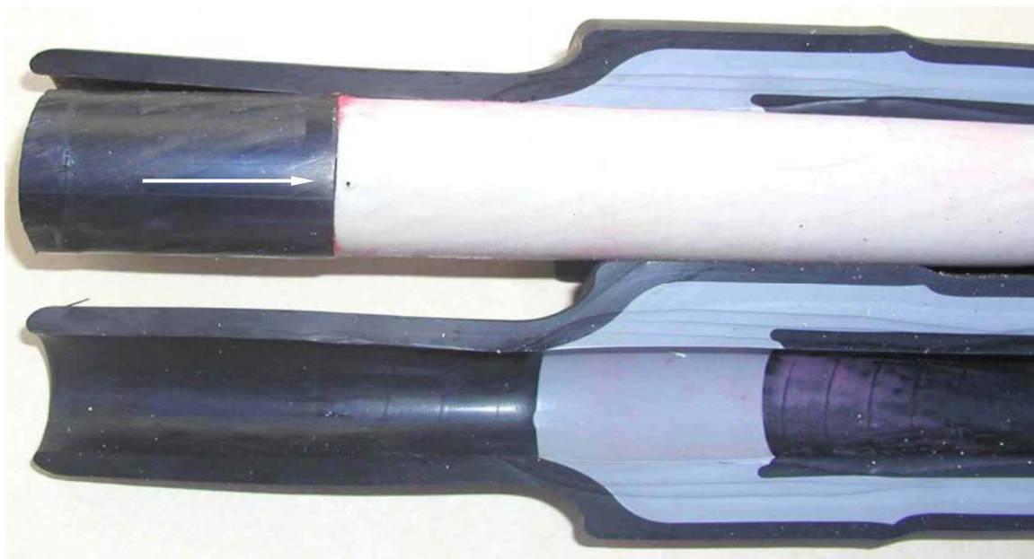
Figure C-2 Joint 3M5. Radial Failure next to the Insulation Shield Cut Back.
