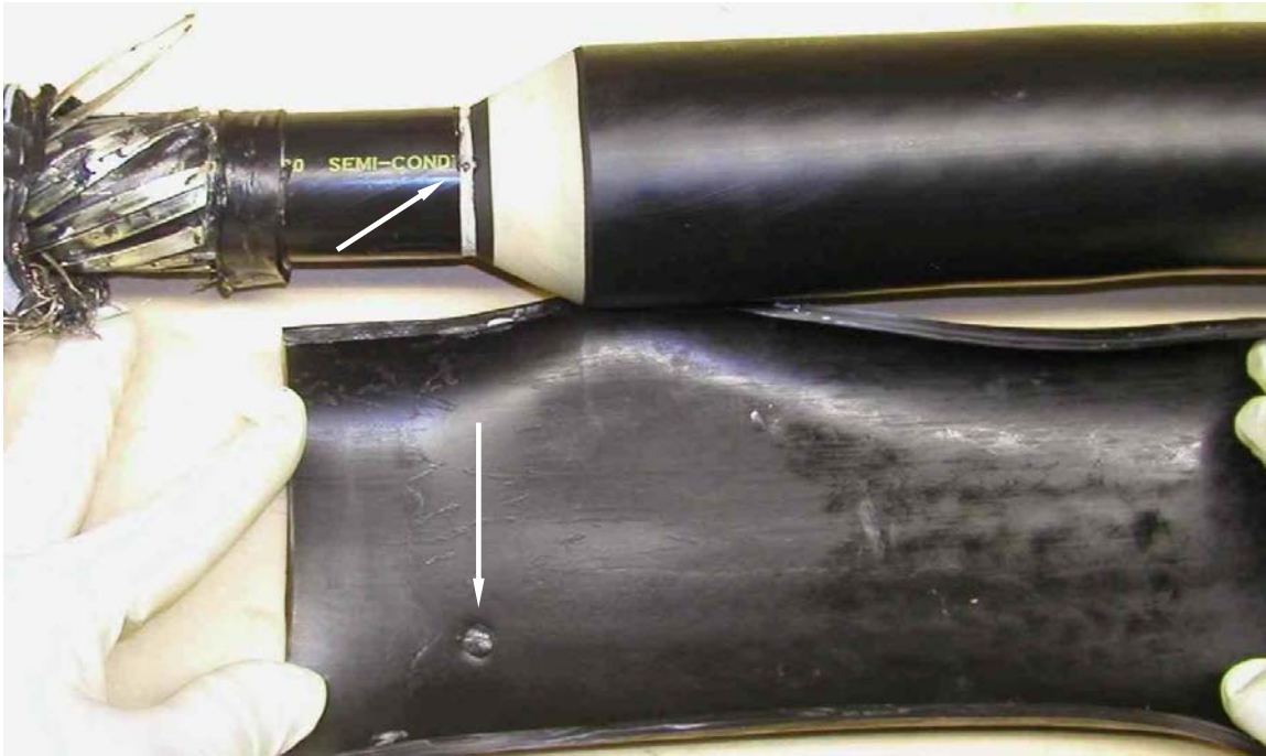
Figure B-1 Joint P5. Radial Failure next to the End Step in Insulation Shield.
