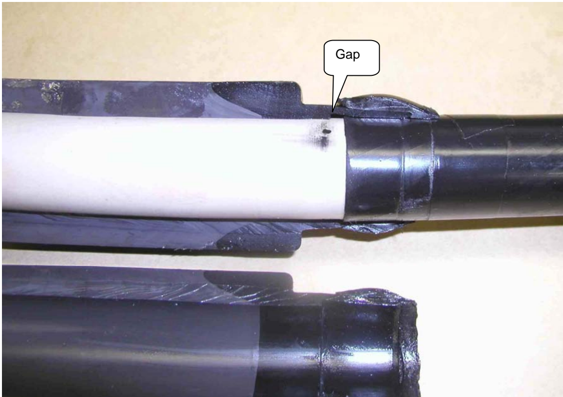
Figure D-5 Joint E3 (with EPR Tape Bumper). Radial Failure at the Step in the Semiconducting Layer of Cable Adapter. Note Gap in this Area.
