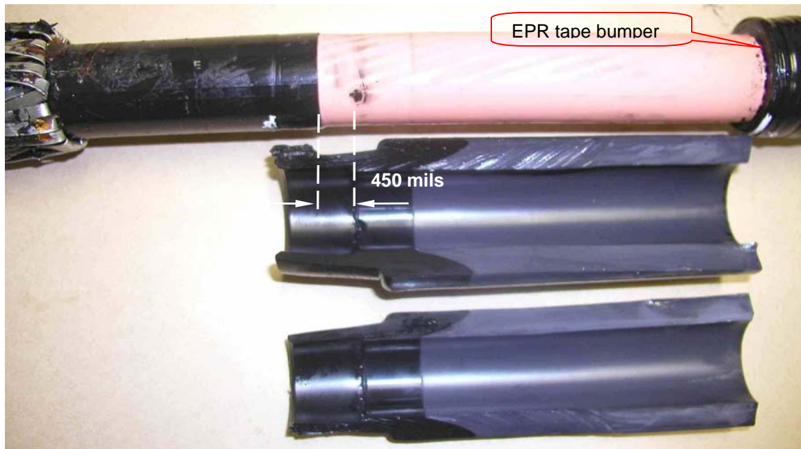
Figure F-3 Joint R5. Radial Failure in Coincidence with the Step in the Semiconducting Layer of the Cable Adapter (About 450 Mils from the Cable Insulation Shield Cut Back).
