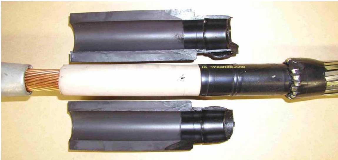
Figure D-2 Joint E1 (with Retaining Ring). Radial Failure at the Edge of Semiconducting Layer of Cable Adapter.
