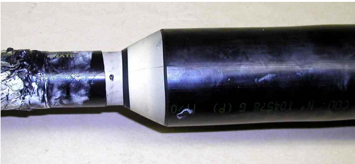
Figure B-2 Joint P2. Radial Failure at 150 Mils from End of Insulation Shield.
