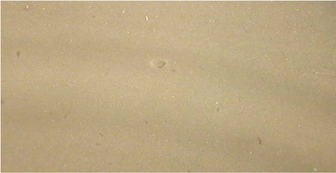
Figure C-5 Joint 3M6. Fifteen Mils Void in Joint Insulation.
