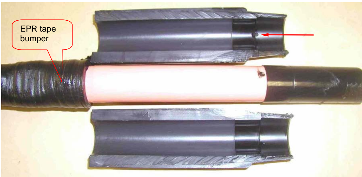
Figure E-2 Joint R6. Radial Failure at the Location of the Step in the Semiconducting Layer of Cable Adapter (90 Mils from the Cable Insulation Shield Cut Back).
