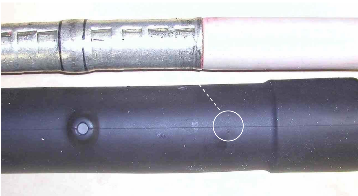
Figure C-4 Joint 3M7. Diagonal Failure next to the Edge of the Connector.
