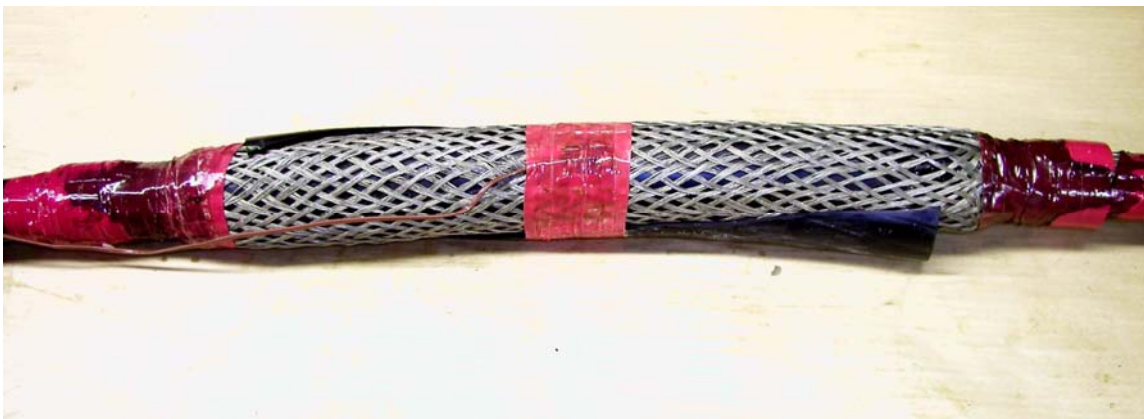
Figure A-4 Split Outer Sleeve of Splice Body in Joint T1 (Heat Cycled in Air).
