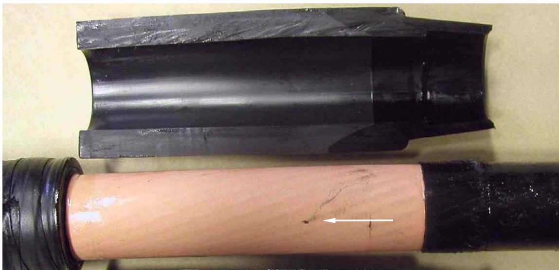
Figure F-4 Joint R3. Radial Failure in the Cable Insulation After Following Longitudinally Along the Interface Between the Insulation of the Cable and the Cable Adapter.
