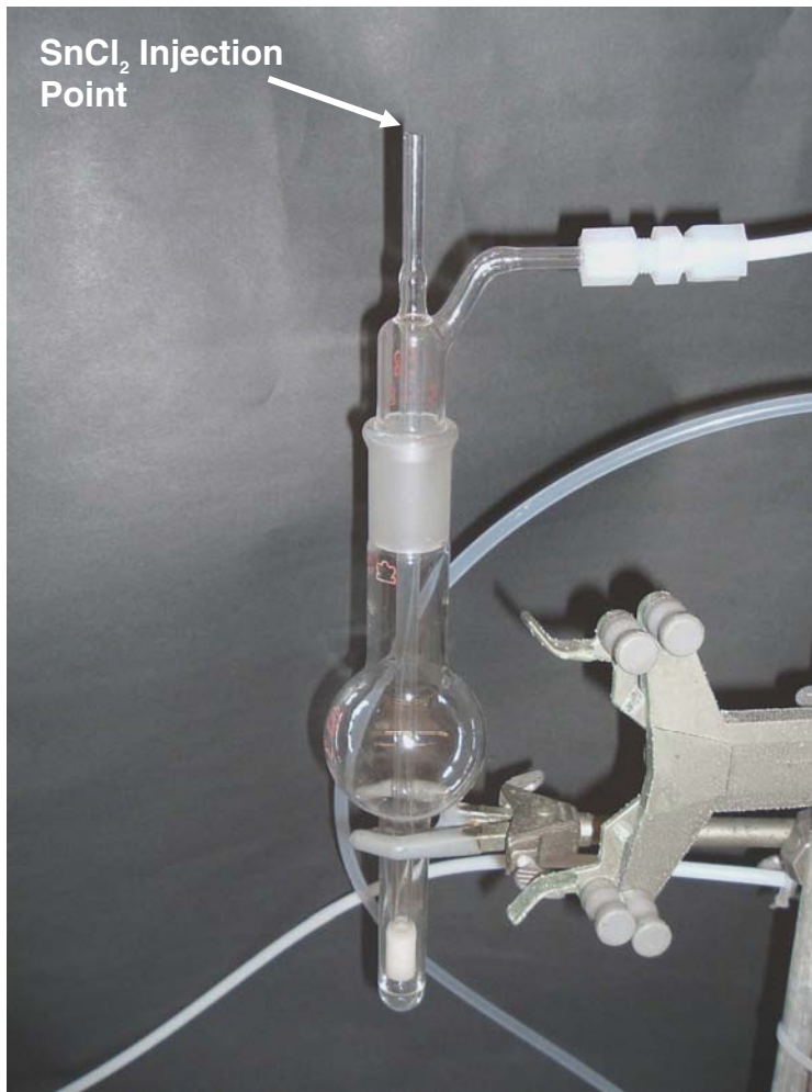
Figure A-4 First impinger stannous chloride injection point
