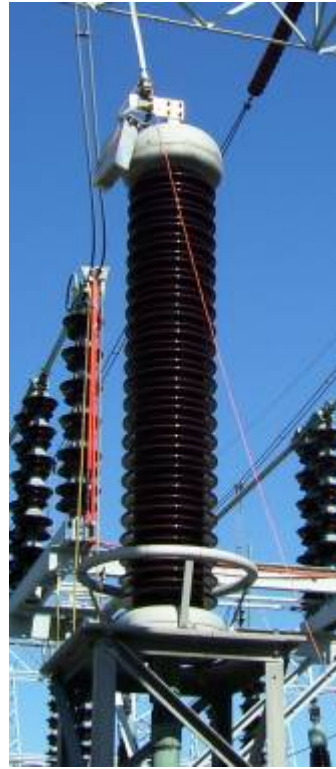
Figure 4-24 Dissipation factor measurement equipment connected to NYPA high voltage bus
