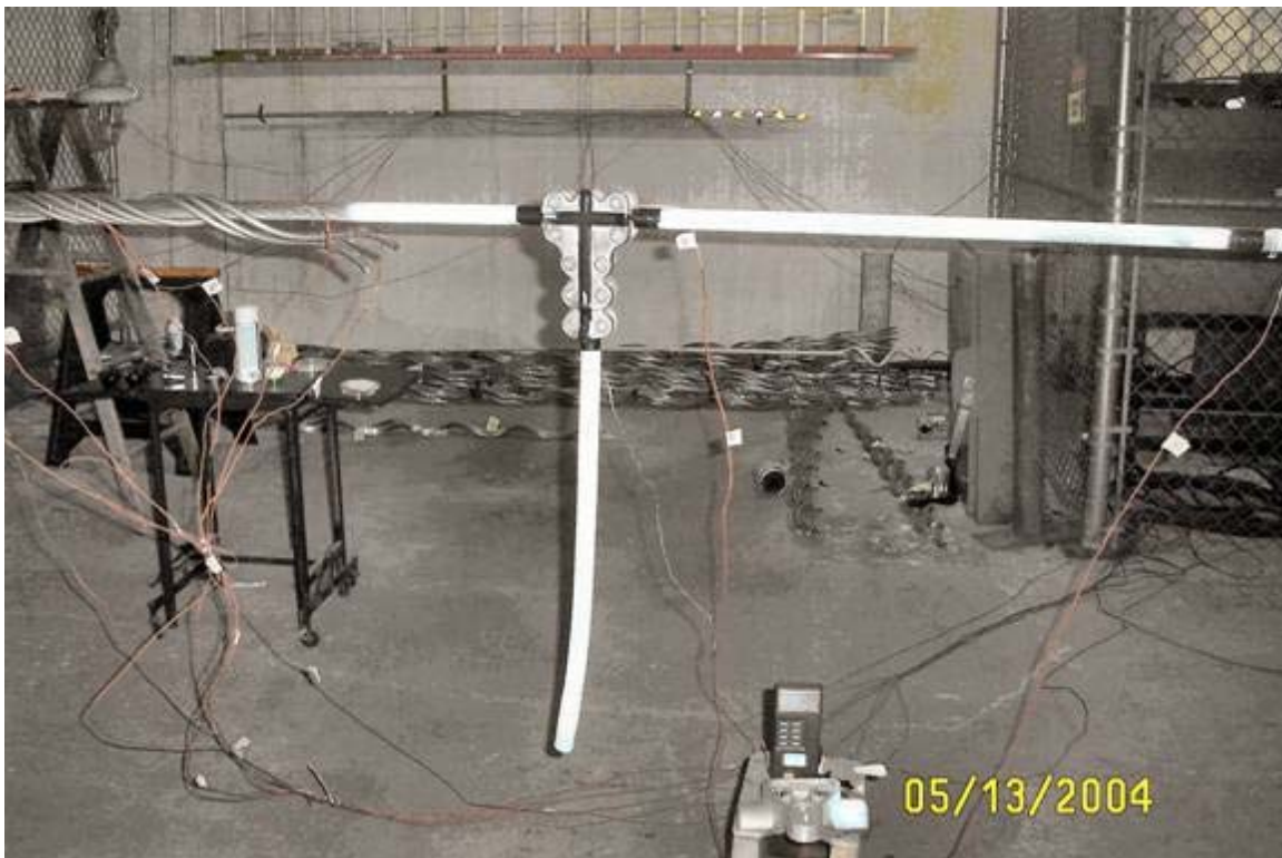
Figure D-10 Pigtail Temperature Gradient Test.
