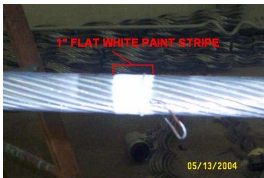
Figure D-8 Painted Target for Distance and Angle Tests
