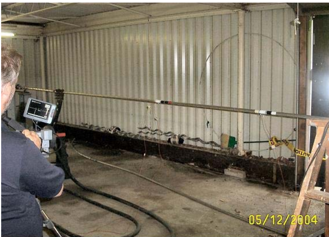
Figure D-1 Laboratory Test Layout Showing Camera and Target.
