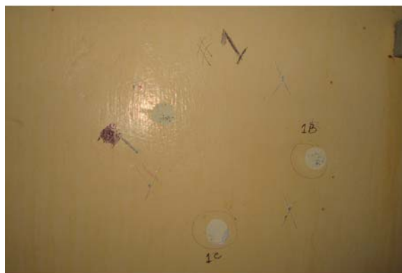
Test Area – With Dolies Removed & Knife Test
