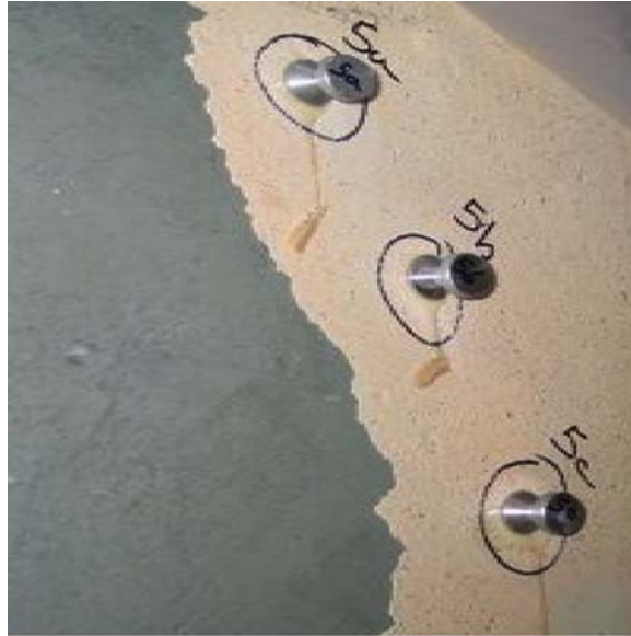
Test Area – As Found with Dollies Installed
