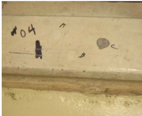
Test Area – Dollies pulled With Knife Test
