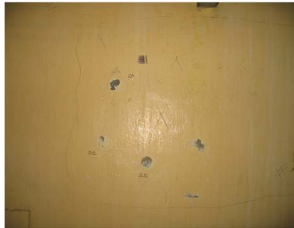
Test Area – With Dollies Removed & Knife Test
