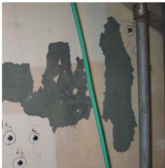
Test Area – As Found with Dollies Installed
