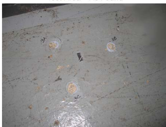
Test Area – With Dollies Removed & Knife Test
