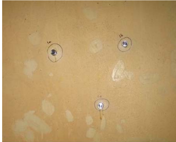
Test Area – As Found with Dollies Installed
