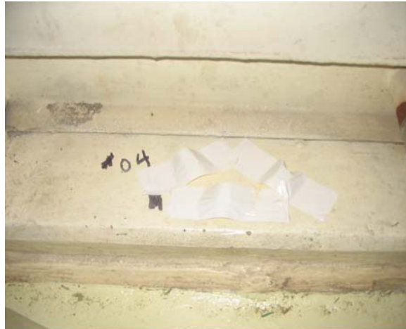
Test Area – As Found with Dollies Installed
