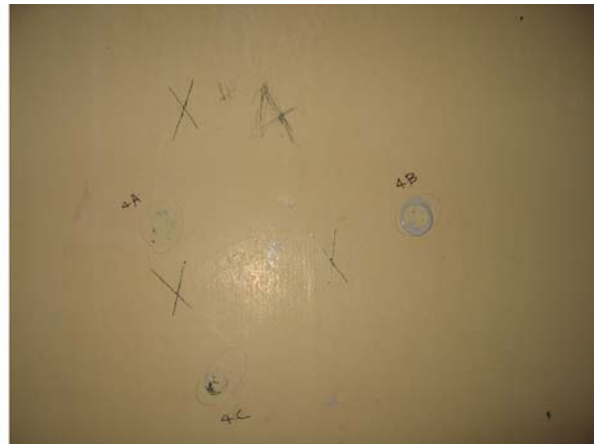
Test Area – With Dollies Removed & Knife Test
