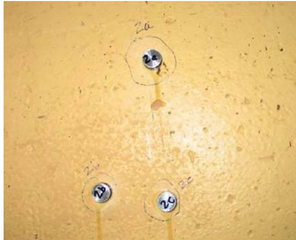
Test Area – As Found with Dollies Installed
