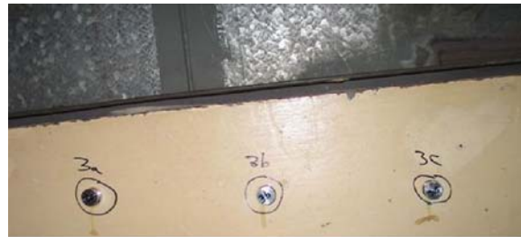
Test Area – As Found with Dollies Installed
