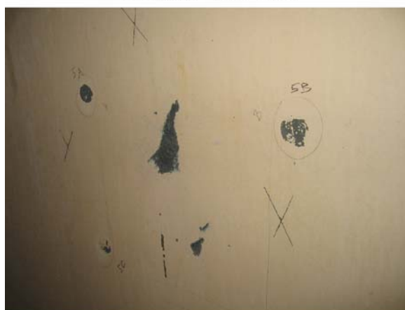
Test Area – With Dollies Removed & Knife Test
