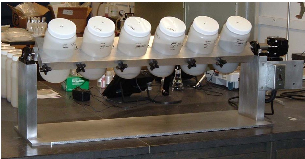
Figure 2-1 Rotary agitation apparatus, driven by gear motor at 28 rpm
