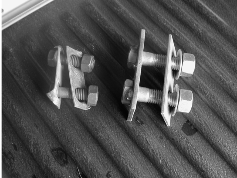
Figure A-7 Before and After Flexible Strap End Bolting (The plate with the stainless steel bolts tack-welded in place provides technicians with a much easier to use bolting configuration.)
