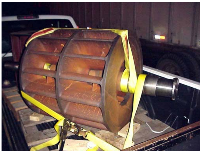
Figure 4-13 Single-Stage Liquid Ring CEU Source: Robinson Nuclear Plant
