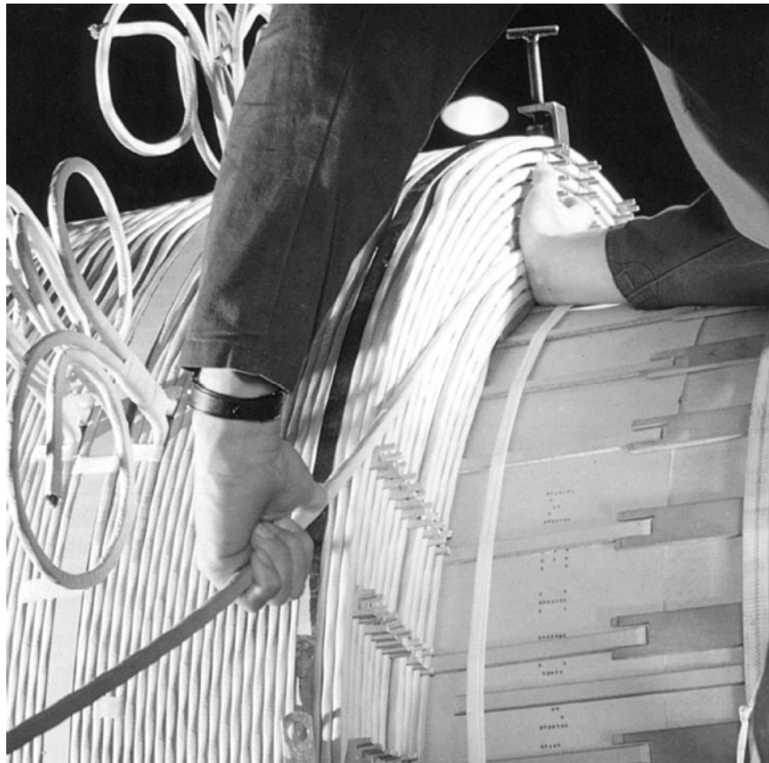
Figure A-10 Construction of Cylindrical Windings Courtesy of Smit
