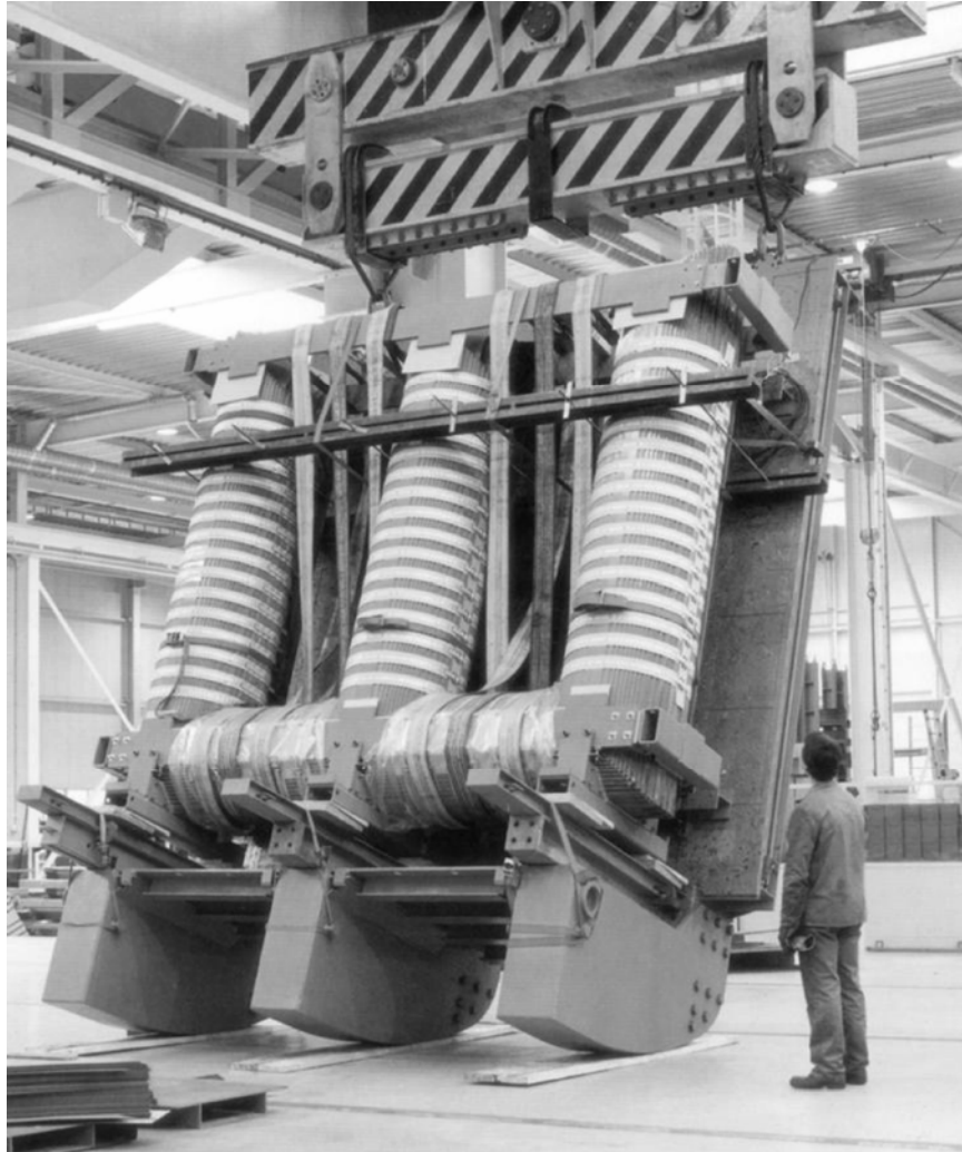
Figure A-6 Clamping of Core Laminations Courtesy of Smit
