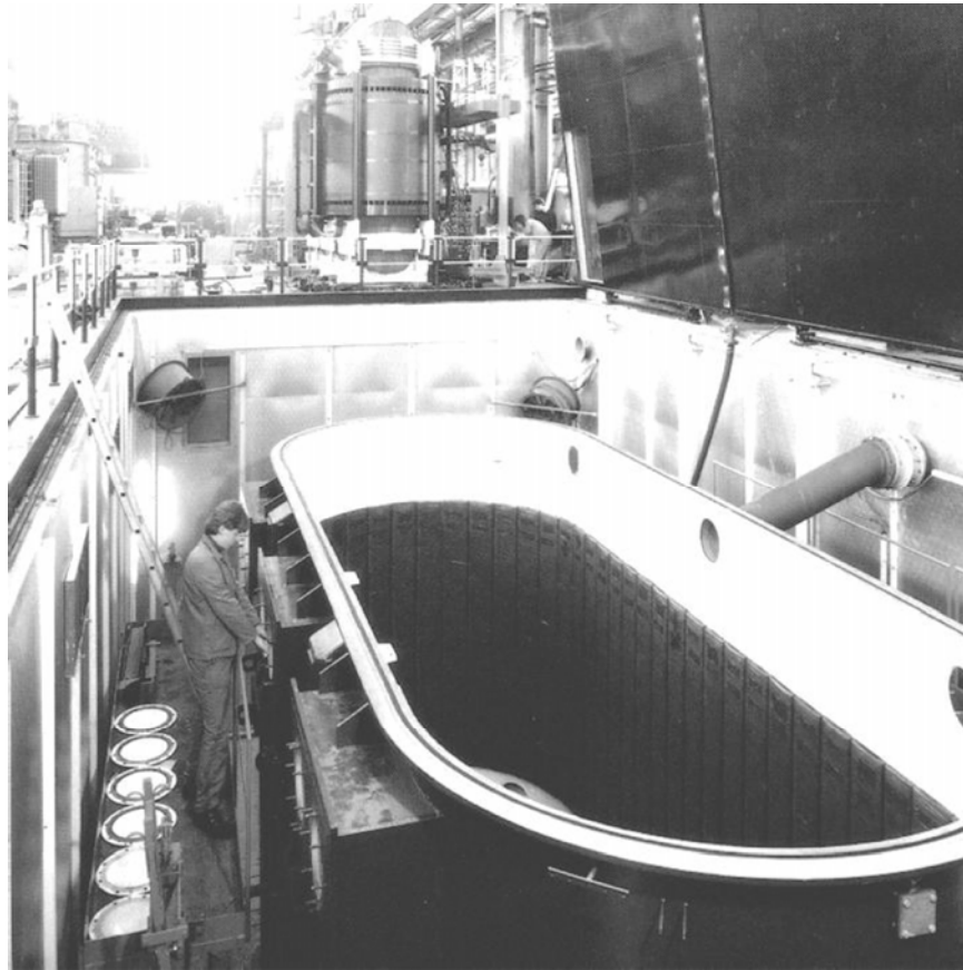
Figure A-1 Typical Transformer Tank Courtesy of Smit
