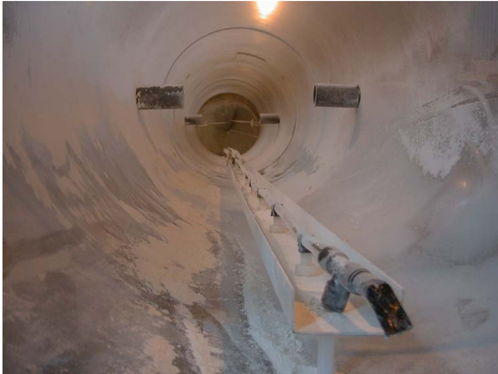
Figure 3-4 Detail of Gas-Injection System and Graphite-Dust Channel
