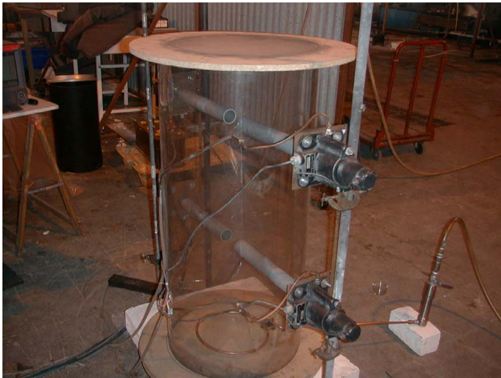
Figure 3-1 CNPP Apparatus for the Determination of the Relationship between Opacimeters and Graphite Dust Concentration
