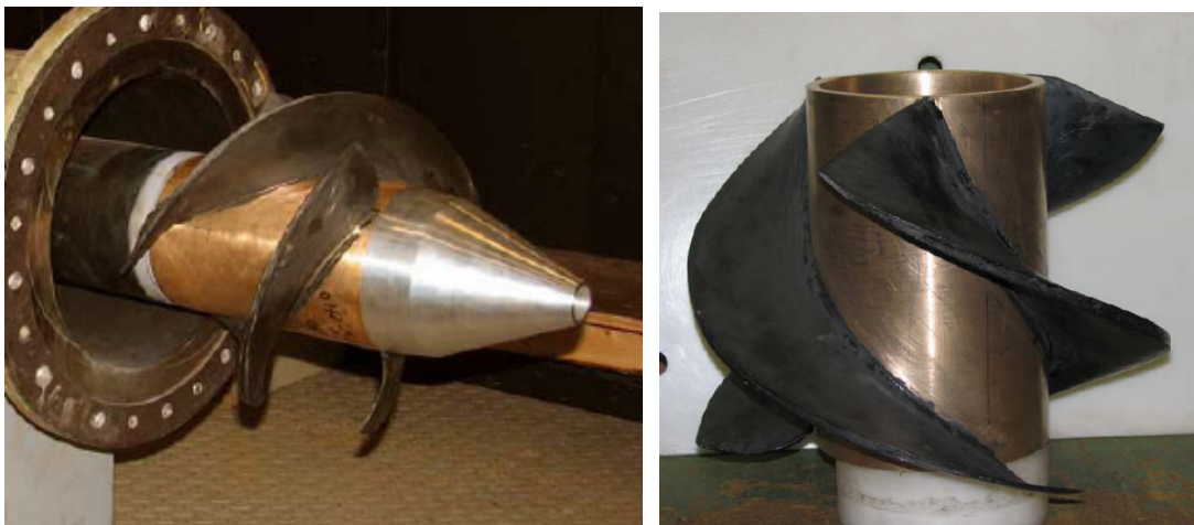
Figure 25-9 Fish-Friendly Turbine Runner Developed by Rapid-Eau, Inc. (de Montmorency 2008)
