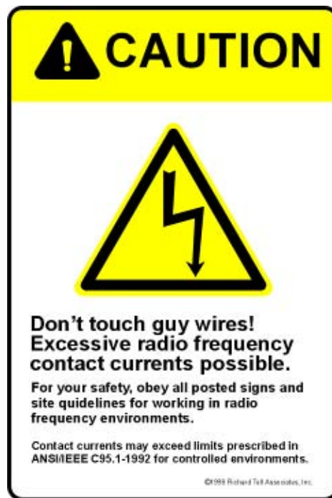
Figure C-5 Caution sign used for alerting personnel to potential for excessive RF contact currents associated with guy wires.
