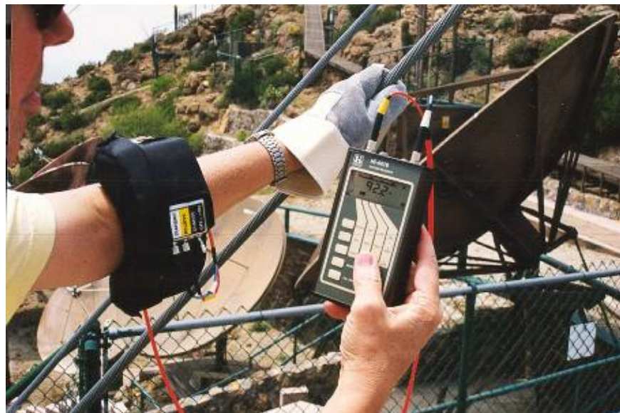
Figure C-4 Evaluating the ability of a leather work glove to reduce contact currents at a VHF/UHF broadcast site found on a tower guy wire. The measured contact current of 92.2 mA (slightly less than the IEEE MPE for contact current in a controlled environment) with the glove was unchanged when the glove was removed and the wire was grasped barehanded.
