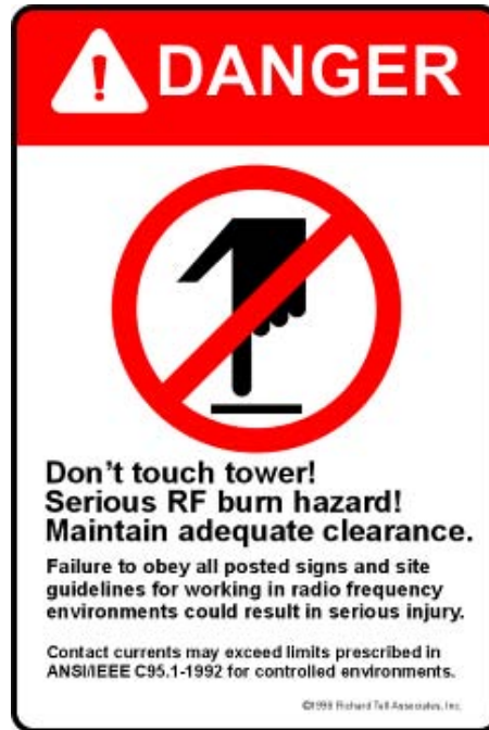
Figure C-6 A danger sign normally used at the base of AM radio towers to alert persons of the potential for an RF burn.
