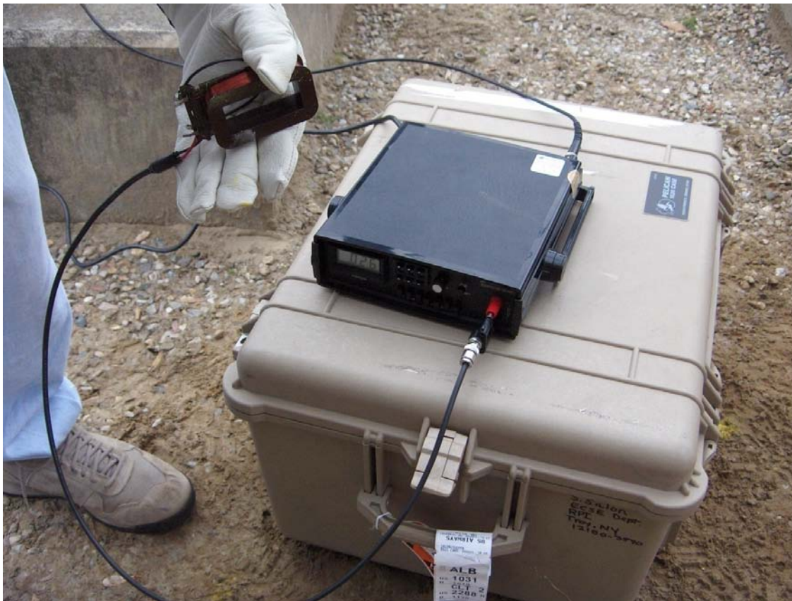
Figure 3-2 Gaussmeter used for detection of the voltage induced in the pickup coil
