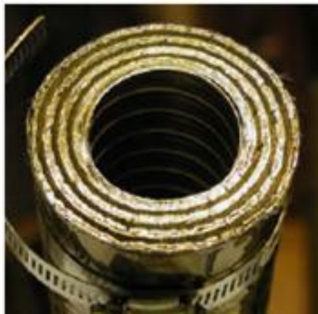
Figure 3-6 Tri-axial HTS Cable Arrangement to be Used for Project HYDRA
