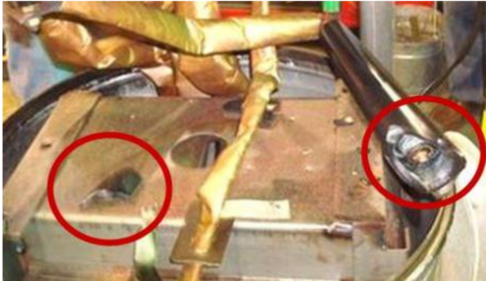
Figure 3-32 Failed Internal Transformer Bushing
