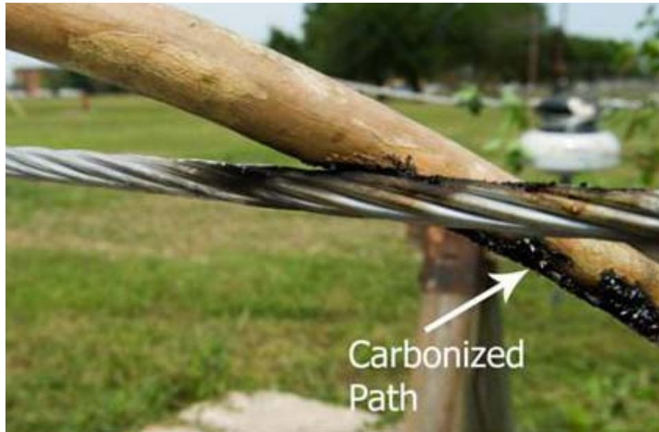
Figure 4-6 Carbonization, or “Char,” Created when Vegetation Bridges Conductors
