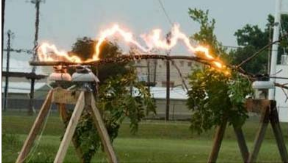
Figure 4-8 Arcing Rising with Hot Plasma and Forming Jacob's Ladder
