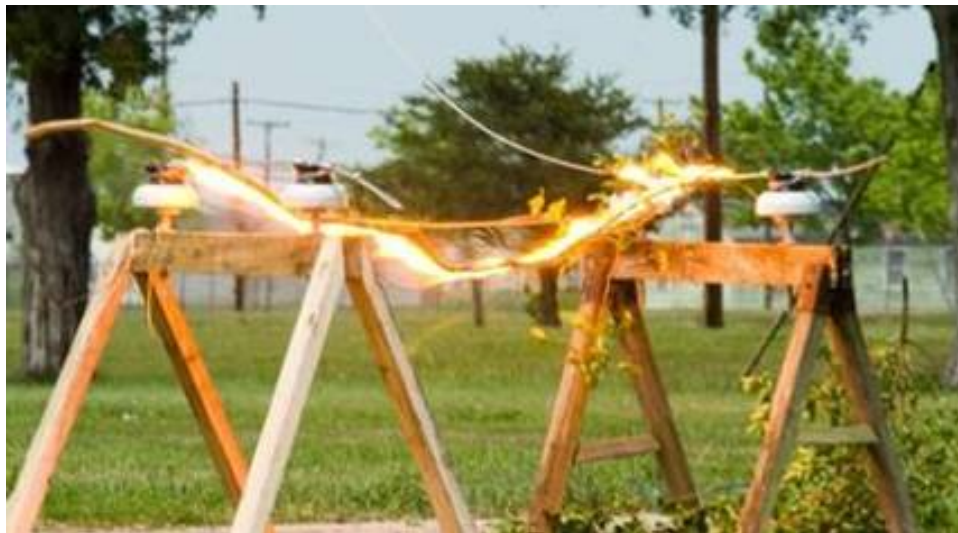
Figure 4-7 Arcing and Burning of Tree Limb Bridging Two Conductors
