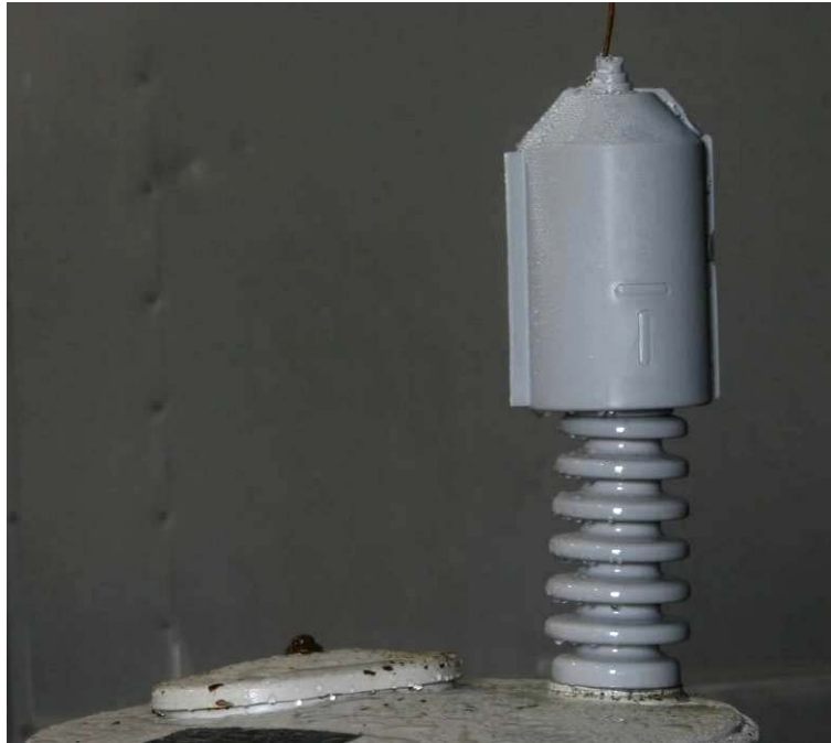
Figure A-12 Wildlife Guard from Sample Set Q Installed on a Test Fixture
