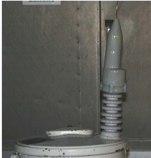
Figure A-9 Wildlife Guard from Sample Set N Installed on a Test Fixture
