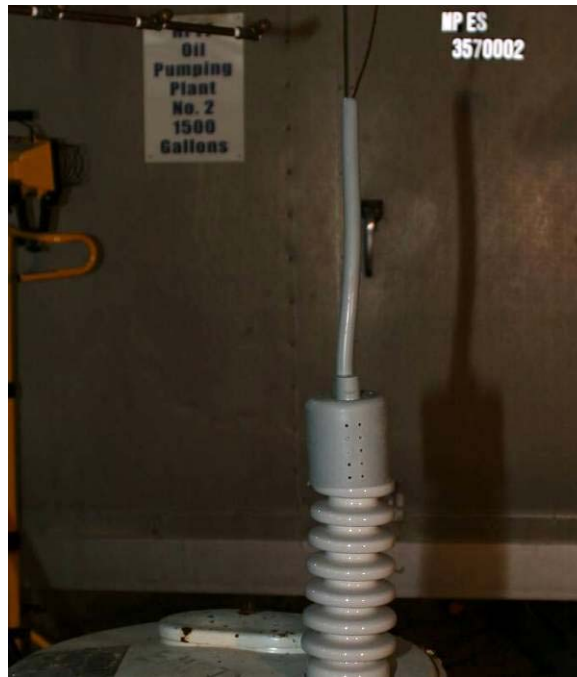
Figure A-10 Wildlife Guard from Sample Set O Installed on a Test Fixture
