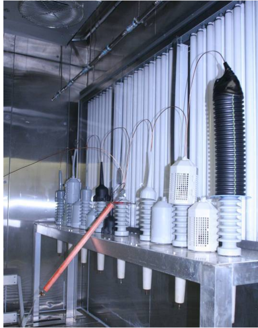
Figure 2-3 Interior of the Multi-Stress Aging Chamber Showing Samples Installed for Testing
