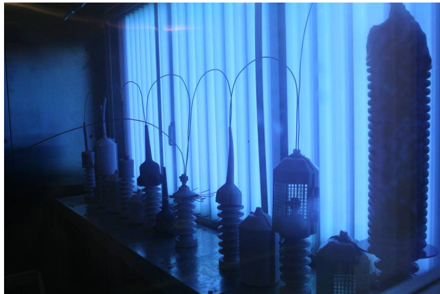
Figure 2-4 Interior of the Multi-Stress Aging Chamber during the Ultraviolet Light Exposure Portion of the Test Cycle
