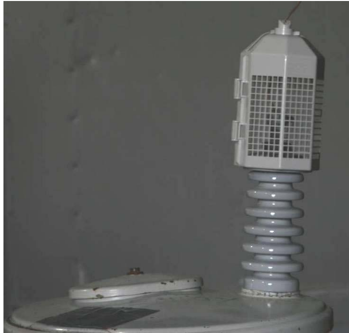
Figure A-5 Wildlife Guard from Sample Set J Installed on a Test Fixture
