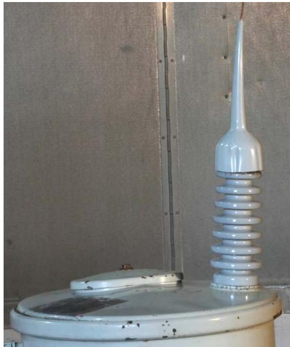
Figure A-2 Wildlife Guard from Sample Set G Installed on a Test Fixture
