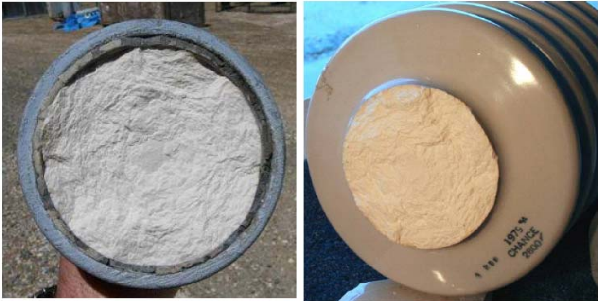
Figure 2-1 Fracture Surface where the Energized End Broke Away from Sample #1: Endcap (left) and Insulator Body (right)
