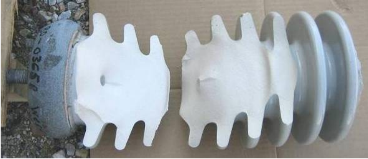
Figure 2-3 Fracture Surface at the Ground End of Sample #1
