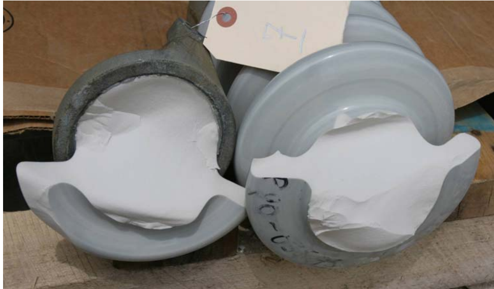
Figure 2-14 Fracture Surface of Sample #7 where the Energized End Trunnion Cap was Broken from the Sample
