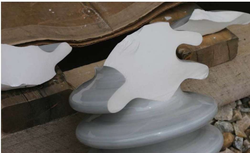
Figure 2-15 Fracture Surface of Sample #7 along the Insulator Body
