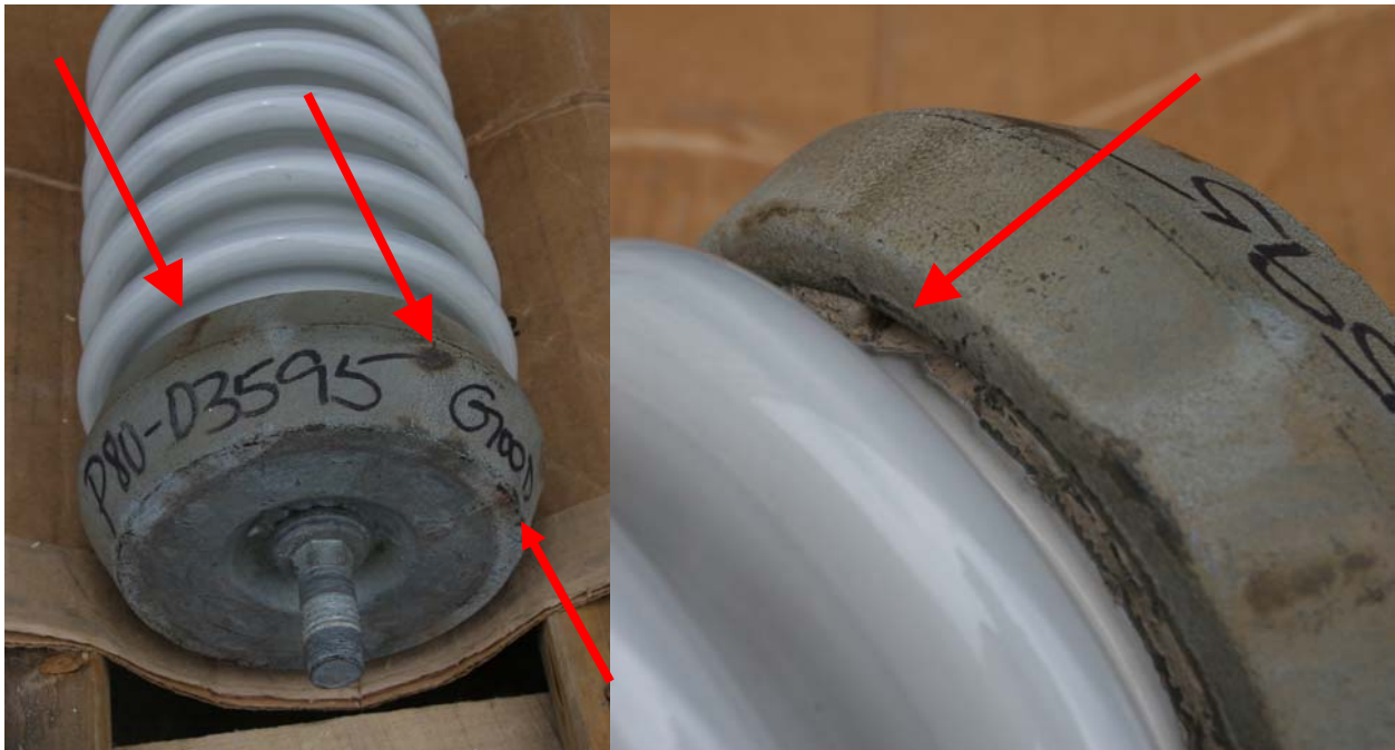
Figure 2-13 Sample #7 Showing Marks on Base End Cap and Small Section of Missing Cement around Base End Cap
