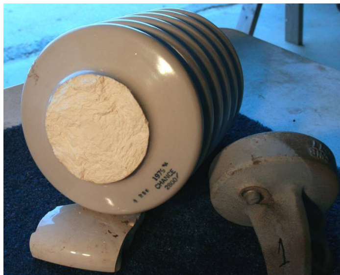
Figure 1-2 Sample #1 Arrived at the Test Facility with the Energized End Broken-Off
