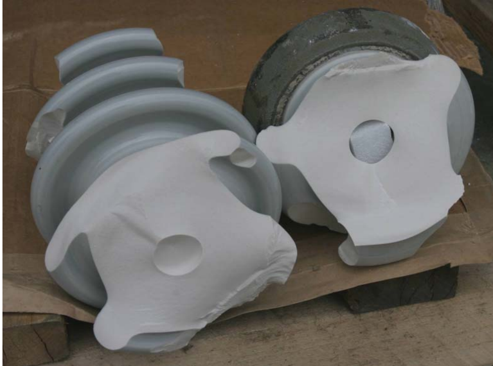
Figure 2-16 Fracture Surface of Sample #7 where the Base End Cap was Broken from the Insulator Body (note that the polystyrene cube in the chucking hole is a normal part of the manufacturing process)
