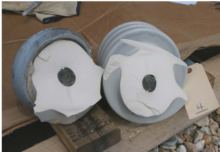
Figure 2-12 Fracture Surface of Sample #4 where the Base Cap was Broken from the Insulator Body
