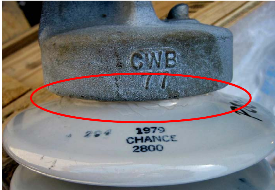
Figure 2-4 Sample #2 Showed a Region of Finely Divided Cracks Just Below the Trunnion Cap
