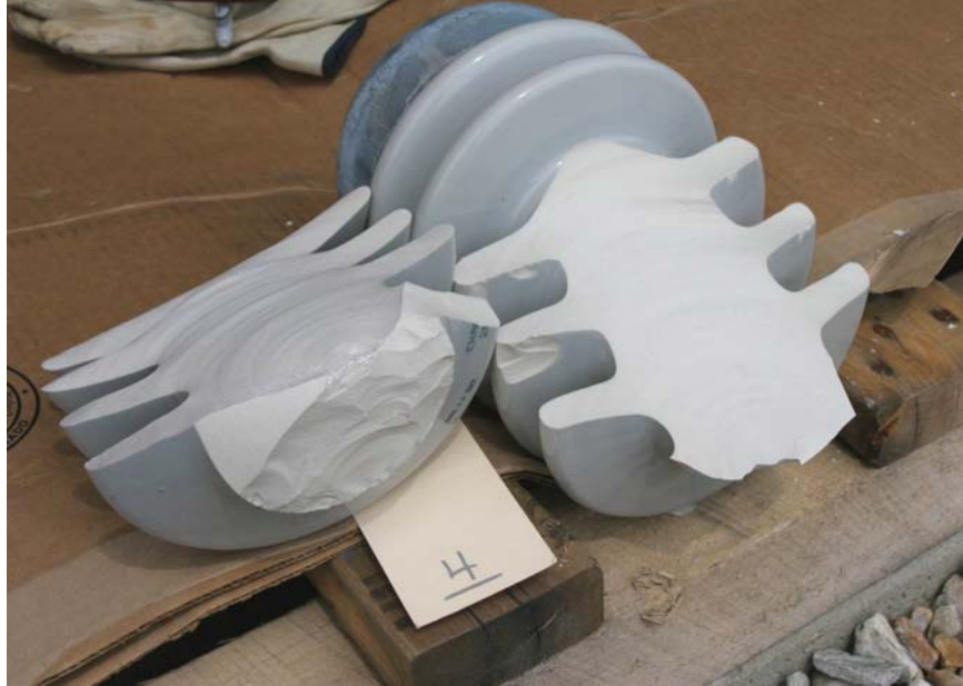
Figure 2-11 Fracture Surface of Sample #4 along the Insulator Body
