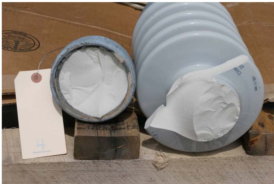
Figure 2-10 Fracture Surface of Sample #4 where the Energized End Trunnion Cap was Broken from the Sample
