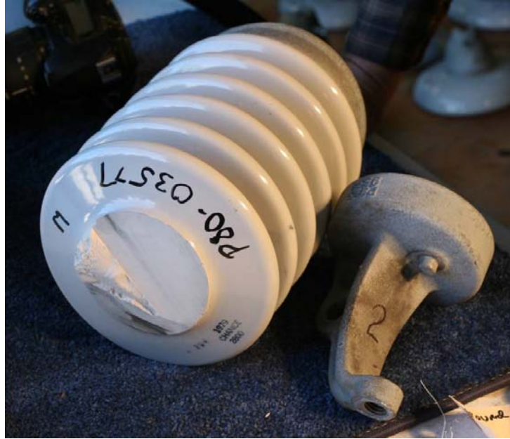
Figure 2-6 The Trunnion Cap was Cut from the Energized End of Sample #2
