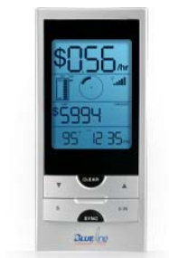
Figure 7-2 Blue Line Innovations PowerCost Monitor for Customer-Side Metering Display
