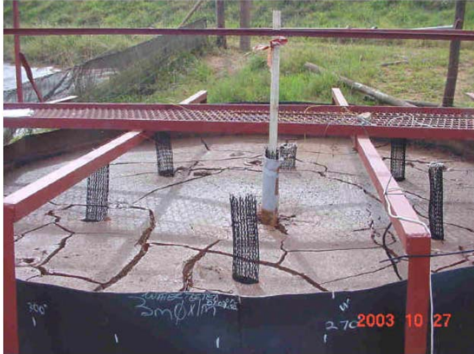
Figure 2-3 Electrokinetics being used to further dewater thickened tailings
