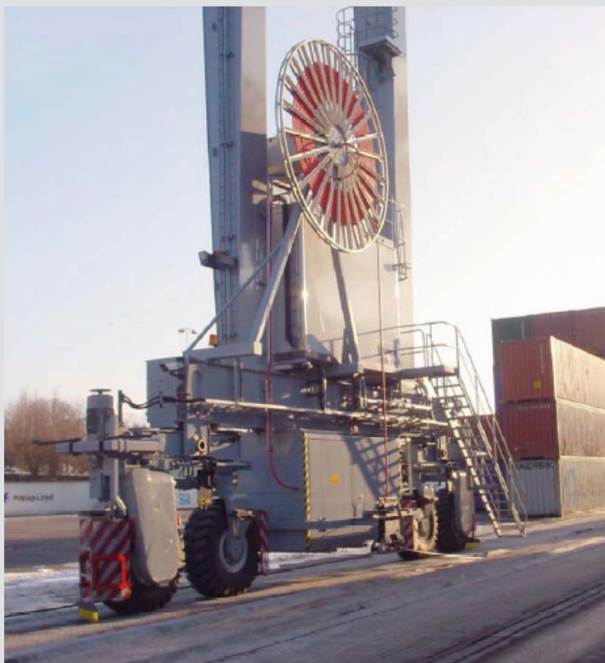
Photo 6: Power cord on a Kalmar Zero Emission RTG (Credit: Kalmar)
