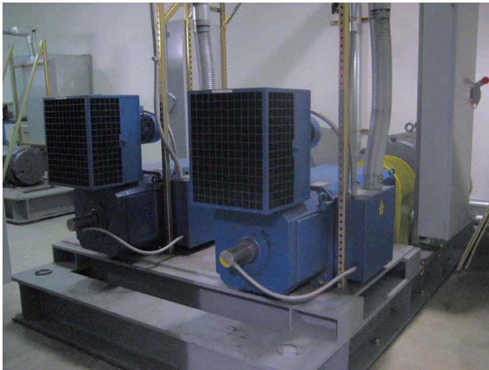
Figure 2-1 Twin DC Motors Used in Testing the AccuSine PCS Active Harmonic Filter
