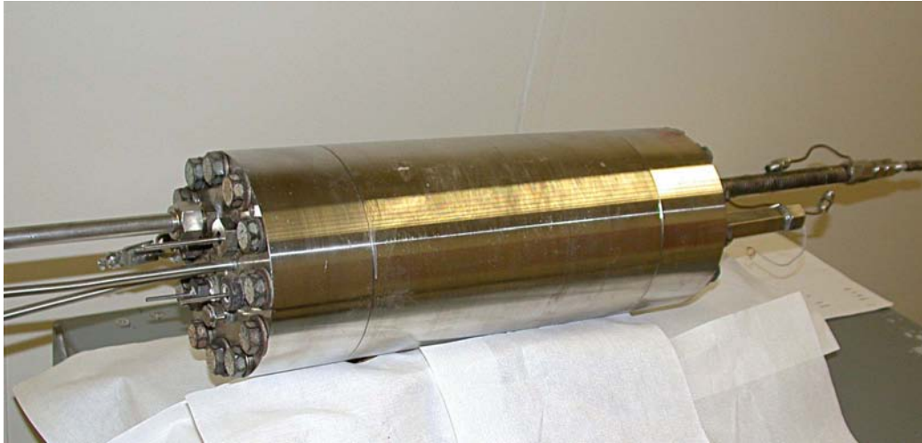
Figure 2-3 Autoclave Immediately After Sealing with Test Solution
