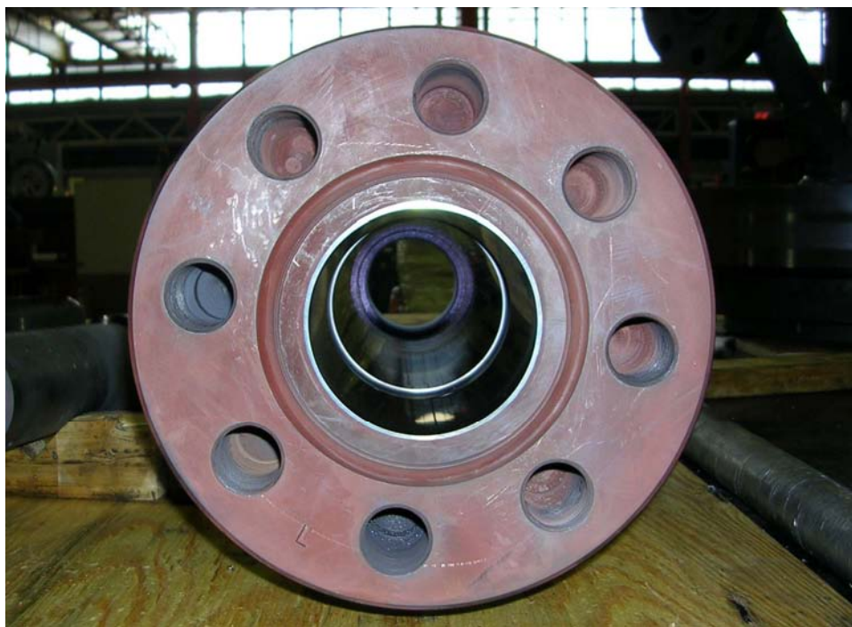
Figure 3-2 Bushing with Stellite sleeve after 8000 hours service with minimal oxide scale
