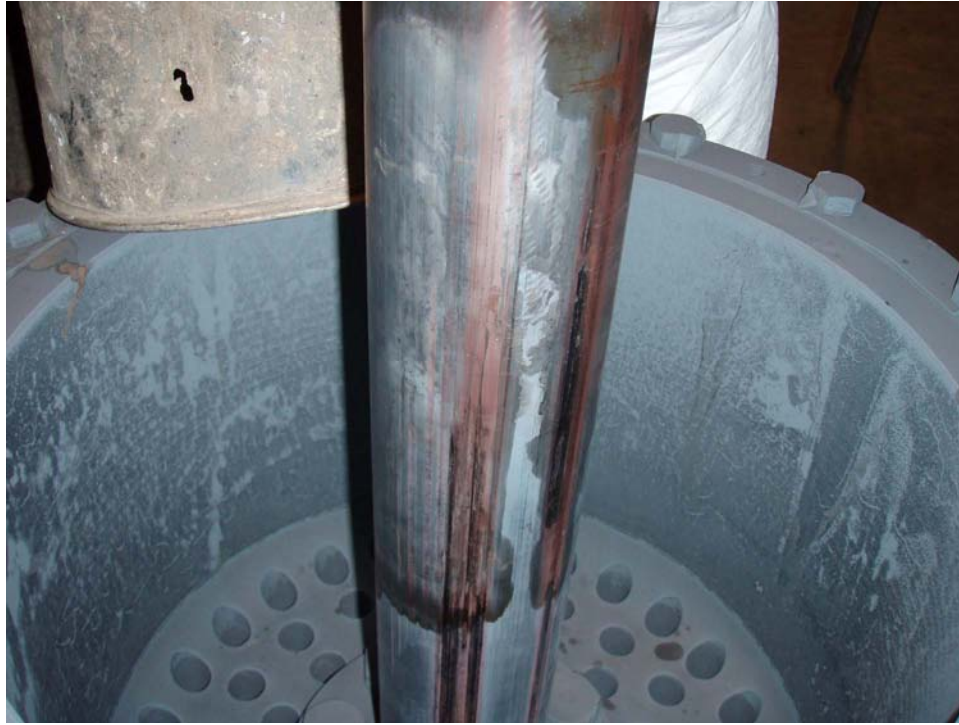
Figure 2-13 Incoloy 901 stem after 48,000 hours of service with minimal oxide scale thickness
