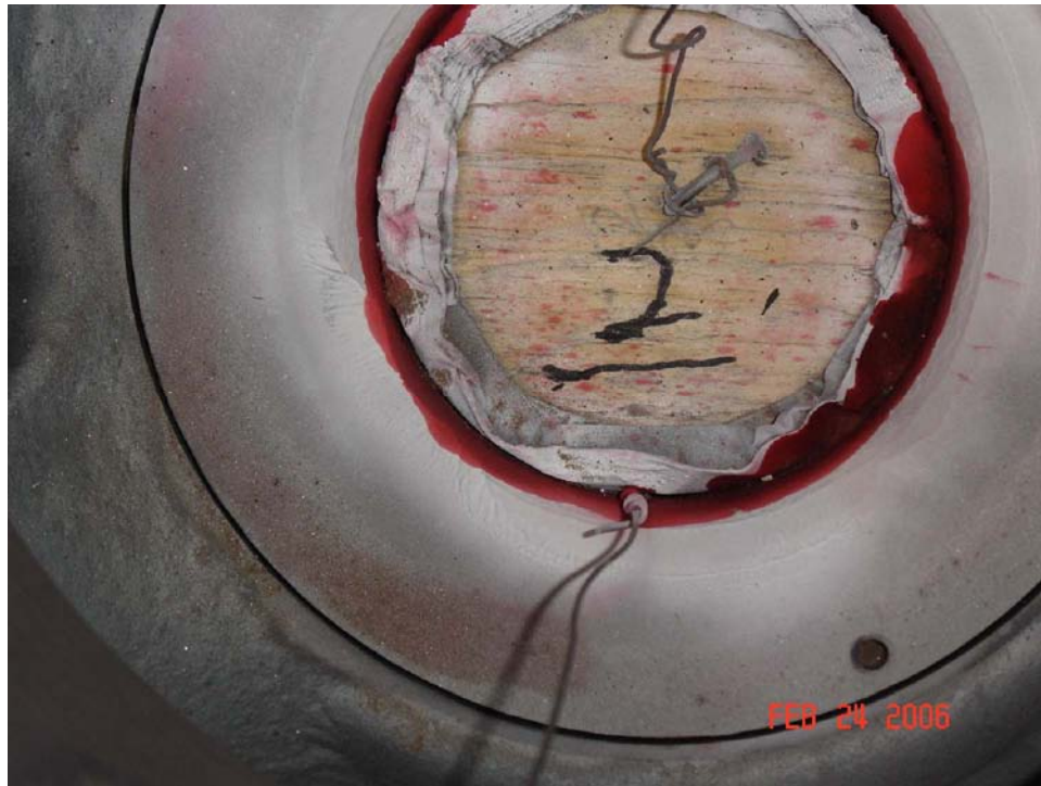
Figure 4-8 Solid particle erosion and transverse weld metal cracks in the Stellite inlay on the seat of control valve 2
