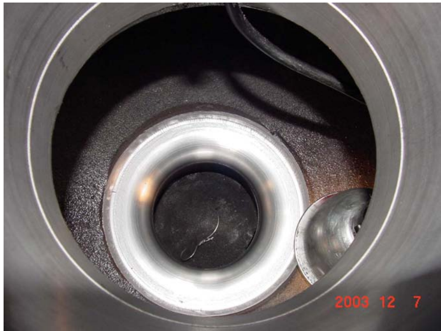
Figure 4-1 Weld-repaired governor valve seat after machining
