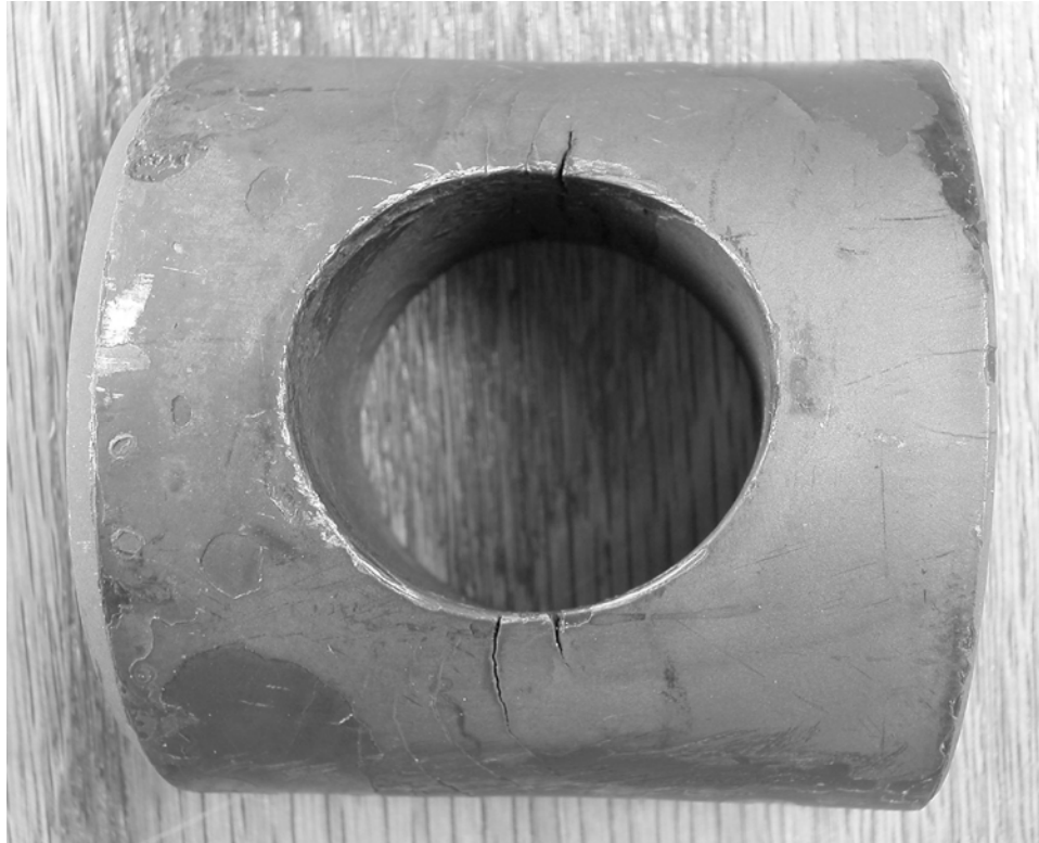
Figure 2-28 Pin hole connection deformation and cracking for a Nitralloy 135M valve stem
