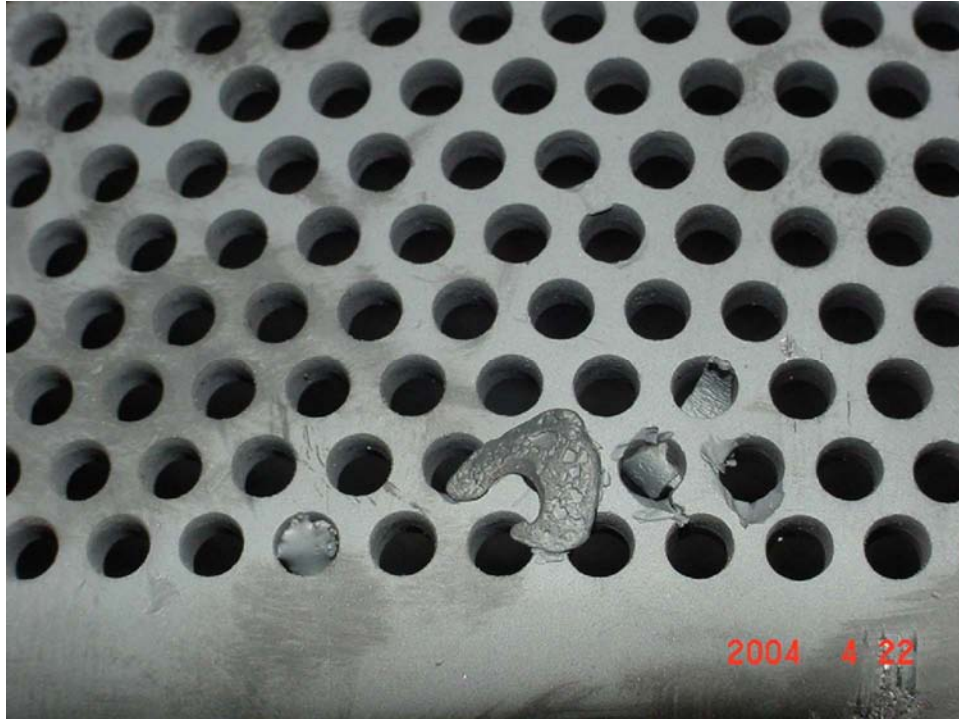
Figure 5-2 Boiler foreign objects caught in a throttle valve strainer
