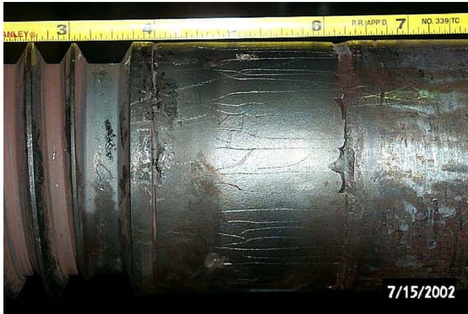
Figure 5-6 Chromium carbide coated (HVOF) stem for a main stop and bypass valve (Courtesy of TVA)
