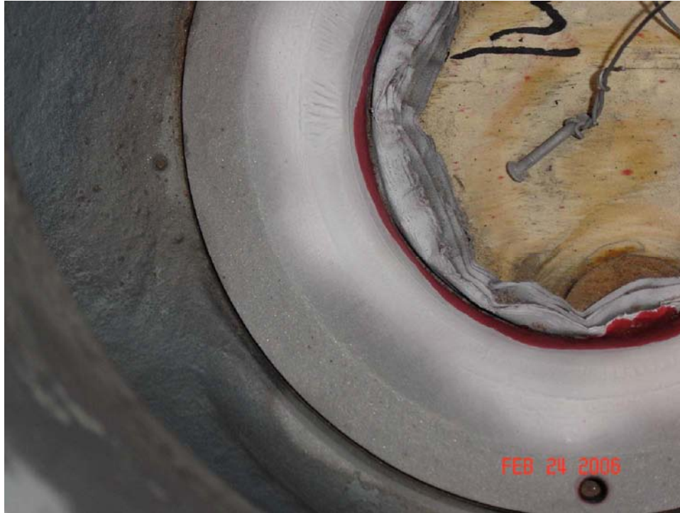
Figure 4-7 Solid particle erosion in the seat of control valve 3
