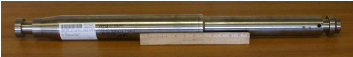
Figure 7-5 Chrome carbide coated Type 422 stainless steel stem (Courtesy of TVA)
