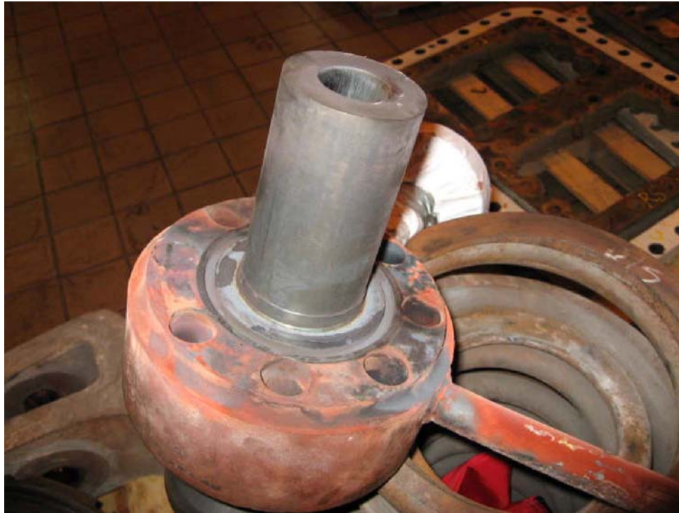
Figure 7-7 Cast solid Stellite 6 bushing (Courtesy of TVA)
