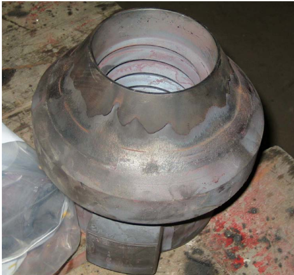
Figure 5-9 Solid particle erosion damage for a General Electric stop valve bypass valve (Courtesy of TVA)
