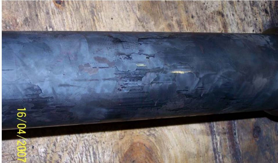
Figure 2-14 Thick and exfoliated oxide scale on nitrided 422 stem
