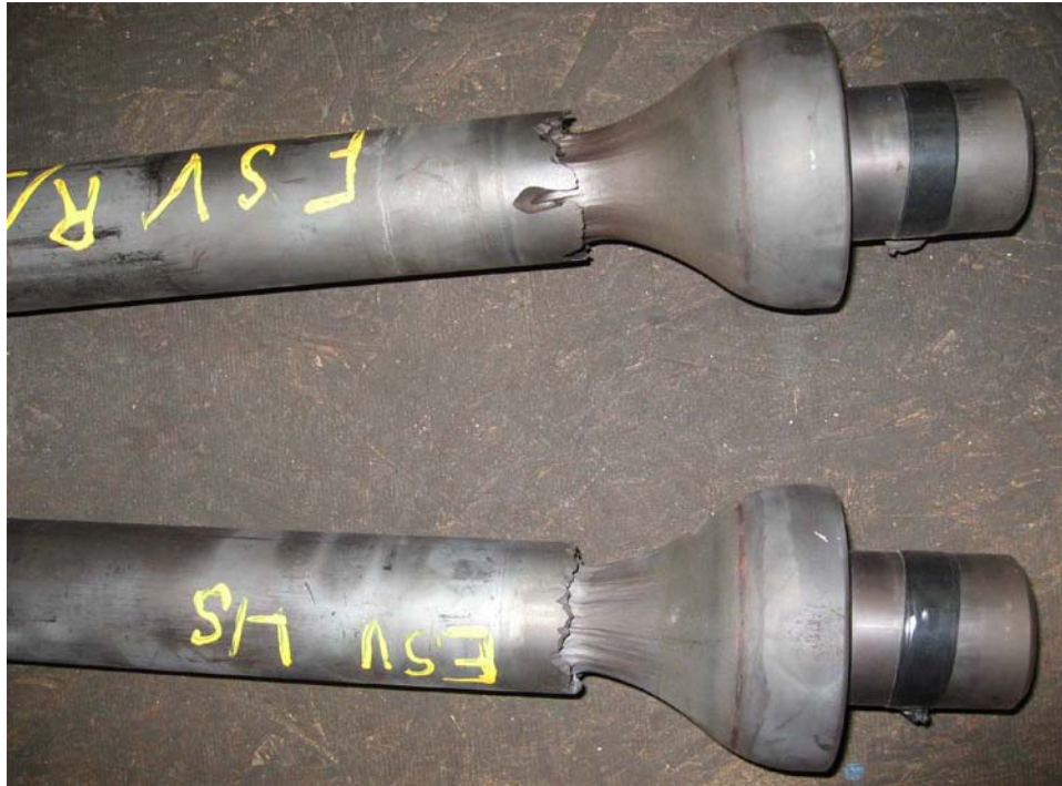
Figure 2-16 SPE damage for two valve stems removed from the ESV at a fossil power plant (Courtesy of TVA)
