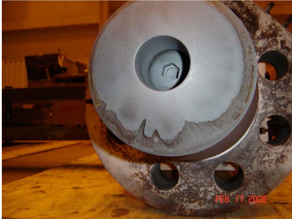
Figure 5-7 Solid particle erosion damage in control valve disc 1 (Courtesy of TVA)
