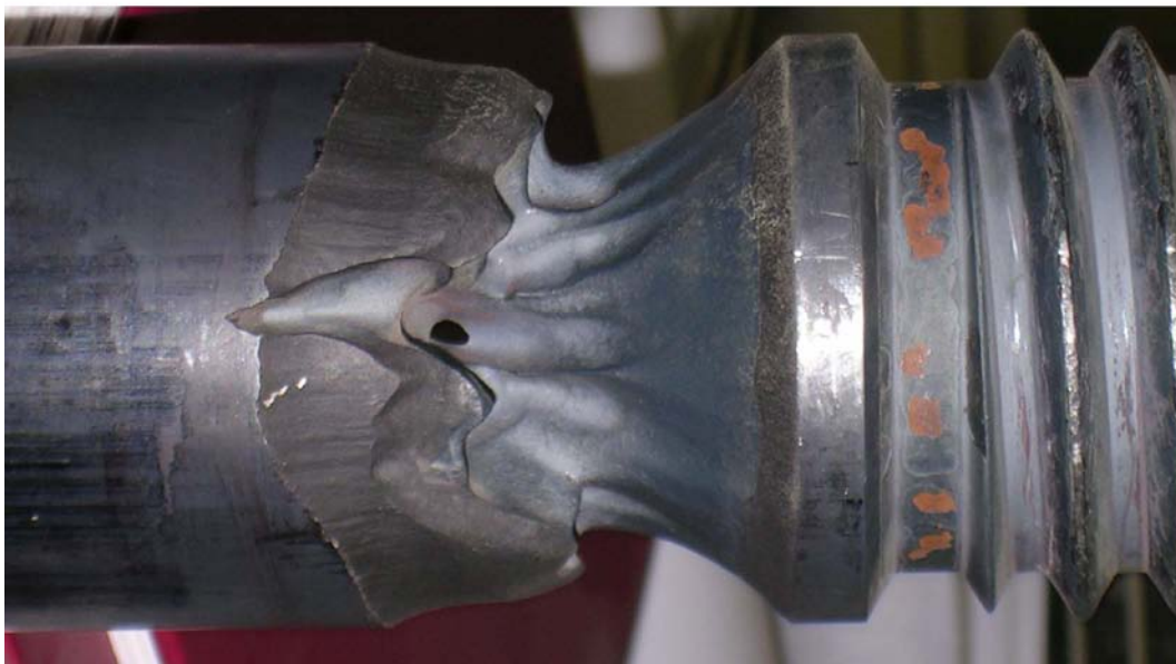
Figure 2-17 Solid particle erosion damage for GE main stop valve stems
