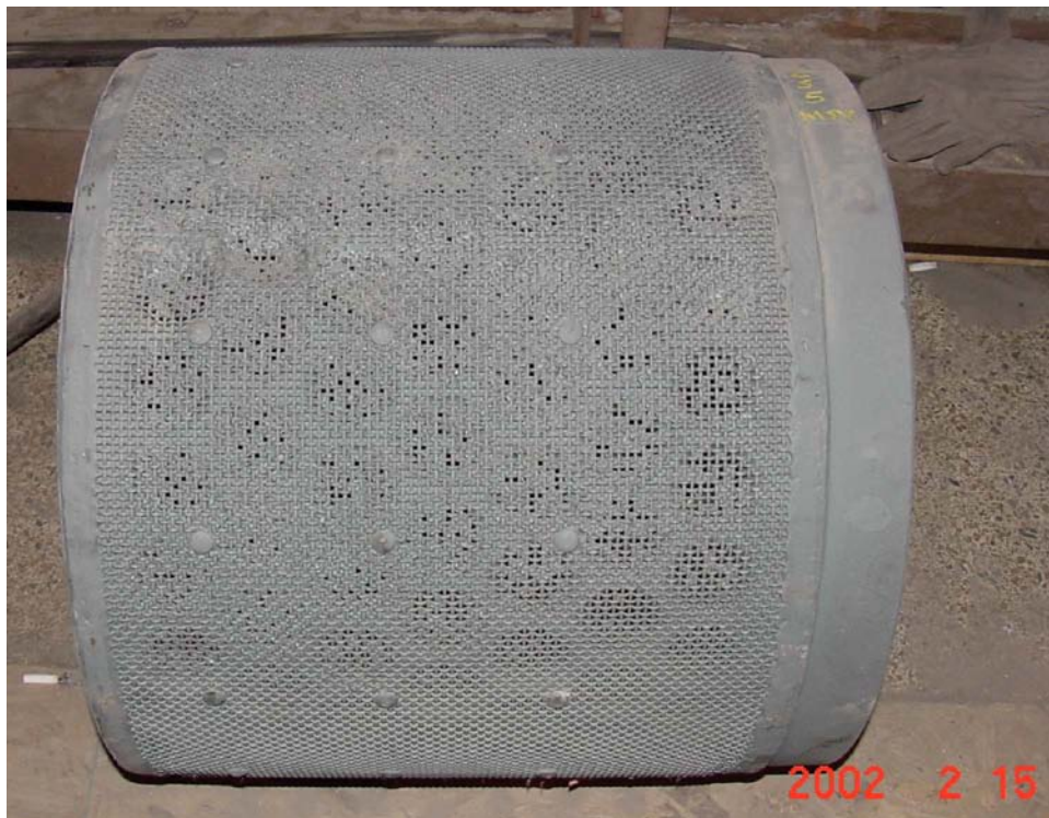
Figure 5-3 Stop valve strainer plugged by an excessive amount of foreign objects and oxide scale
