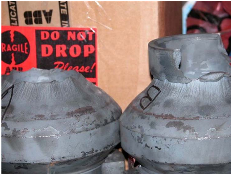
Figure 5-4 Failed discs with significant solid particle erosion damage. The discs were removed from a General Electric main stop and bypass valve. (Courtesy of TVA)
