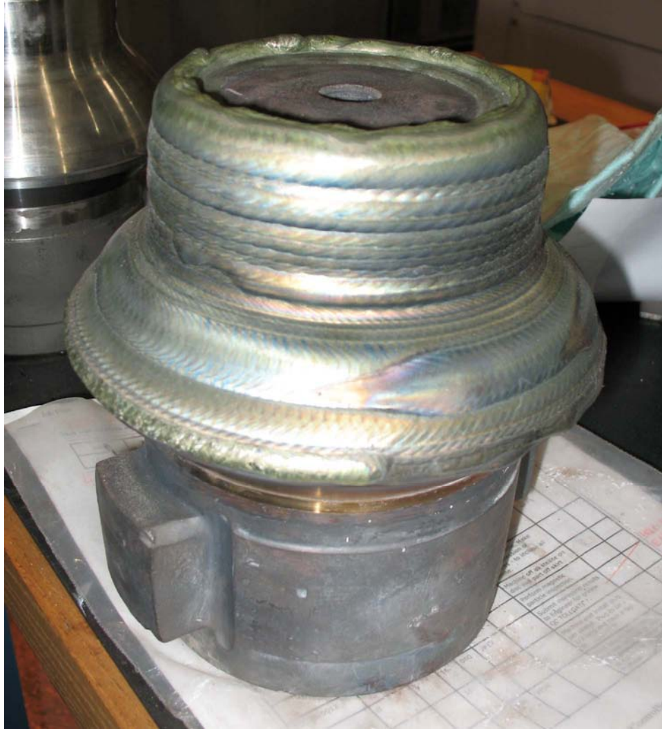
Figure 5-19 Disc with a weld build-up repair
