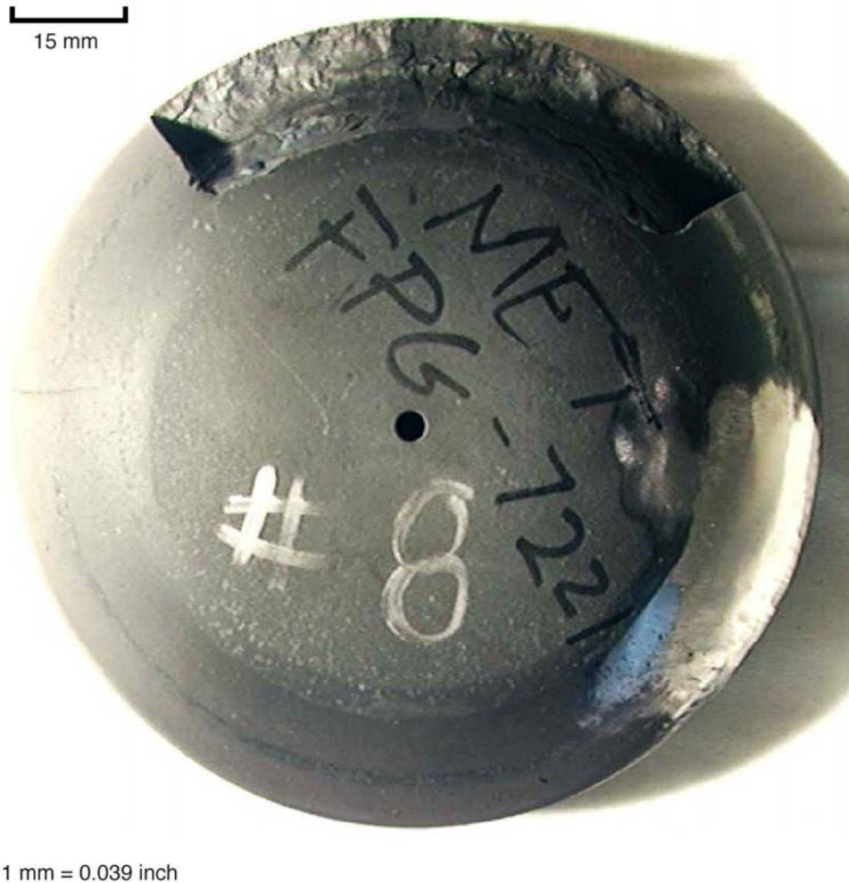
Figure 5-11 Photograph of Stellite weld metal failure for governor valve disc, The sample is shown in as-received condition. (Courtesy of TVA)
