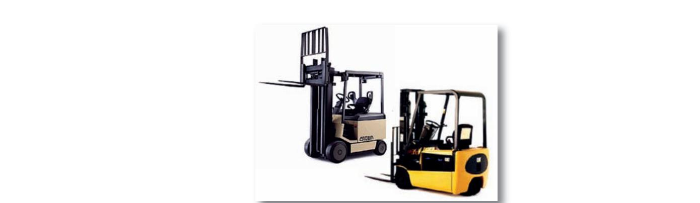
Electric industrial lift trucks provide a quiet, zero-emission, efficient alternative to internal combustion equipment in warehouses, factories and any enclosed areas where forklifts are used.
