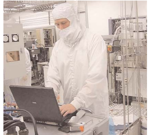
Figure 1. Semiconductor Fabricators Routinely Require Voltage Sag Testing at the OEM Site
