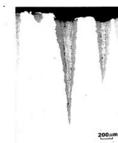
Figure 2-6 Metallographic Cross Section of Circumferential Cracks Showing Typical Sharp Pointed Characteristic and Oxide (Dark) and Sulfide (Light) Deposits (3)
