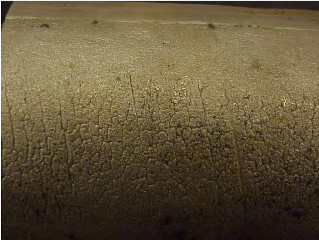
Figure 2-5 Typical Tube Quench Cracking from Spraying Water on Clean Tube Surfaces (1)
