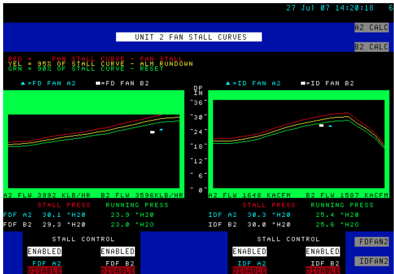
Figure 2-11 Existing GGS Fan Stall Graphic
