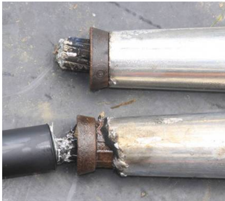
Figure 4-25 The Lower Splice and Conductor Suffered Severe Damage and Probably Would Have Broken Had the Conductor Been Under Tension
