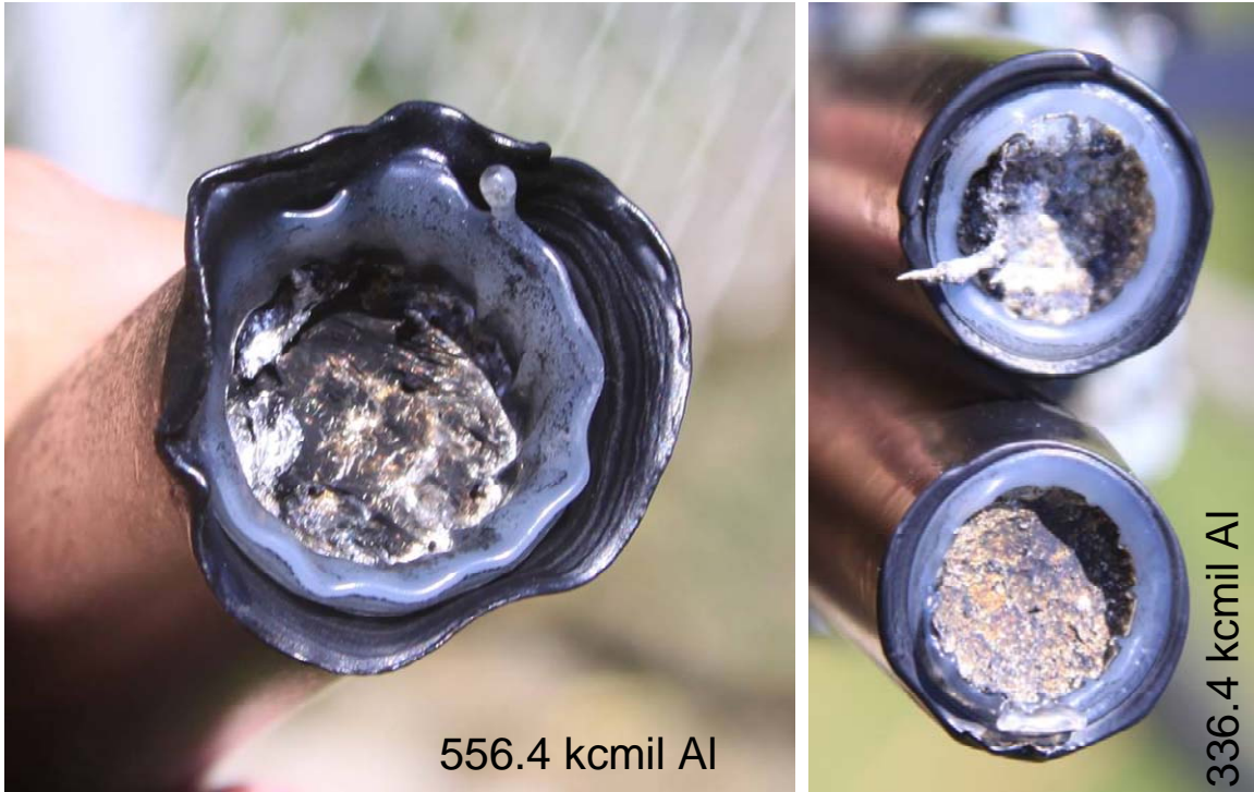
Figure 4-19 The Strands of 556.4-kcmil (281.9-mm 2 ) Aluminum Covered Conductor (Tree Wire) Are Vaporized During a Burndown Event
