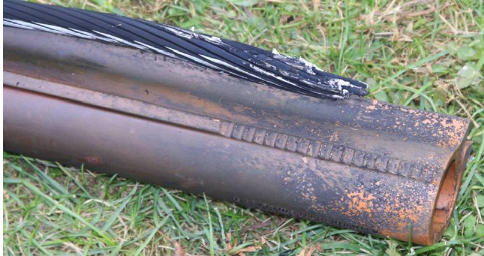
Figure 4-34 Section of 336.4-kcmil (170.5-mm 2 ) Aluminum Conductor After Burndown Event
