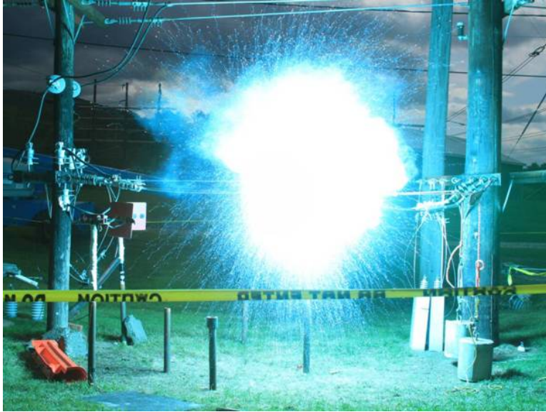
Figure 4-26 Conductor Burndown Test on 336.4-kcmil (170.5-mm 2 ) Aluminum Tree Wire with Automatic Splices
