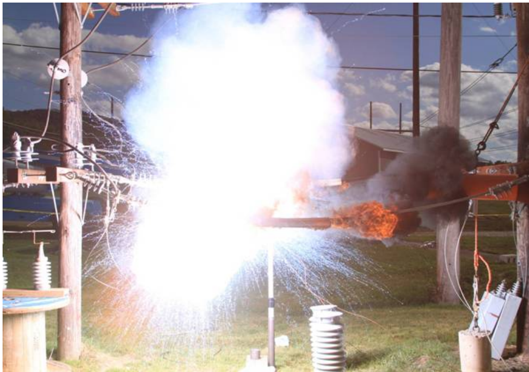
Figure 4-33 Conductor Burndown on 336.4-kcmil (170.5-mm 2 ) Aluminum Conductor at a Line Hose
