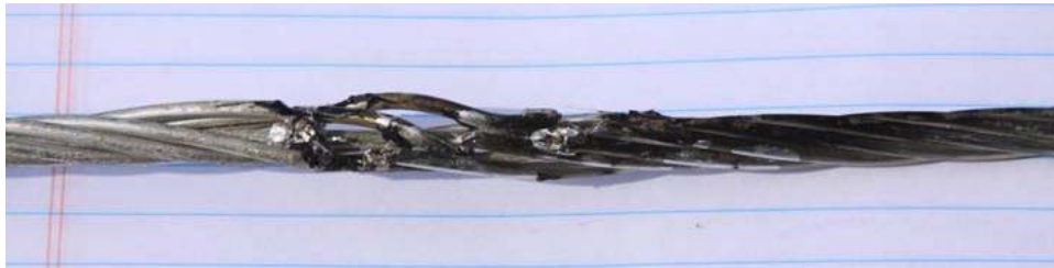
Figure 4-22 This Damaged Section of #4 ACSR Conductor Was Encapsulated in the Jaws of a Vice-Top Polymer Insulator During a Running Arc Test
