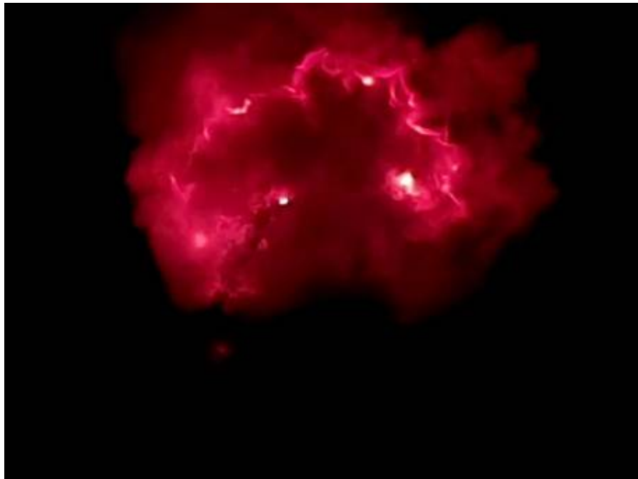
Figure 3-7 One Frame from a 300-Frame-Per-Second Movie of a Burndown Event Taken with an IR Filter
