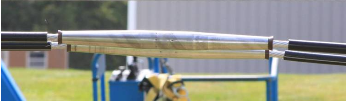
Figure 4-24 Automatic Splices Installed on 336.4 kcmil (170.5 mm 2 ) Aluminum Tree Wire
