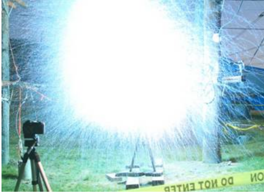
Figure 3-6 Typical View of an Arc Flash Event Using a Camera Recording Visible Light (1/1600 @ f/11, ISO 100)
