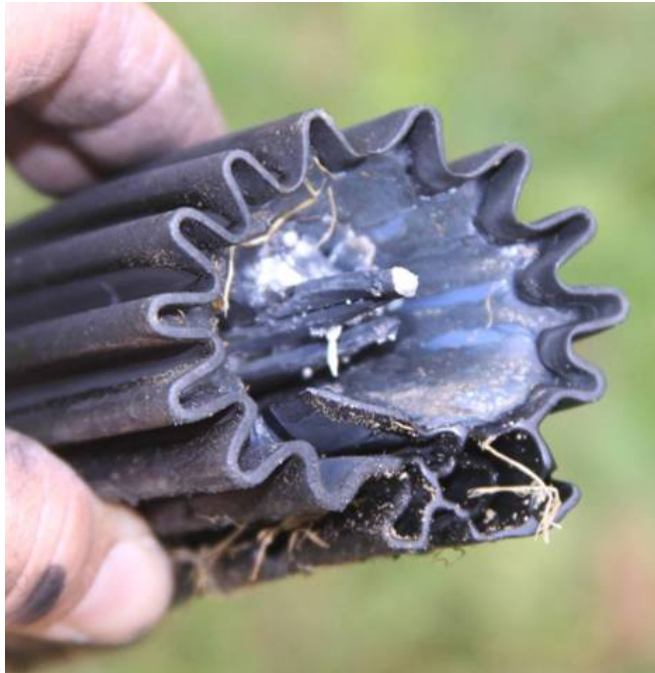
Figure 4-36 Burndown at Gel Wrap on 336.4-kcmil (170.5-mm 2 ) Aluminum Conductor
