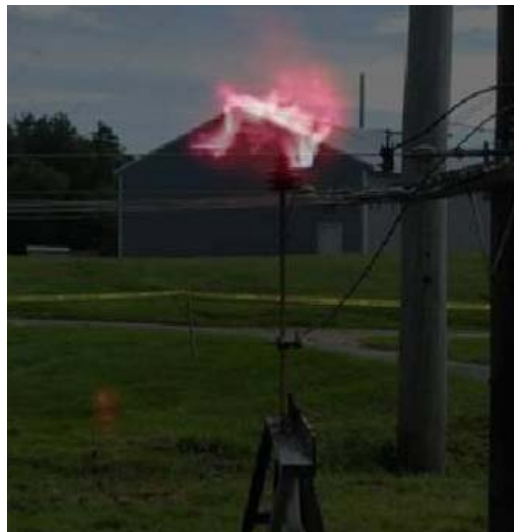
Figure 4-5 Arcs That Remain Relatively Stationary Result in Faster Burndown Times
