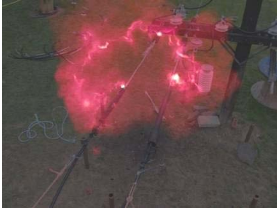
Figure 3-8 Overlaid Composite Image Made from an IR-Filtered Image and a Visible Light Reference Image
