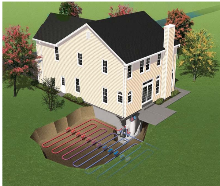
Figure 2-2 Schematic of a Horizontal Ground Loop Heat Exchanger
