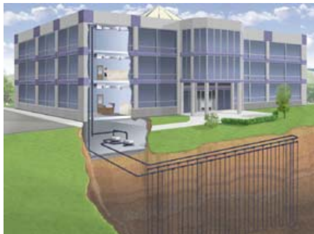
Figure 2-5 Schematic of a Vertical Bore Heat Exchanger in a Building
