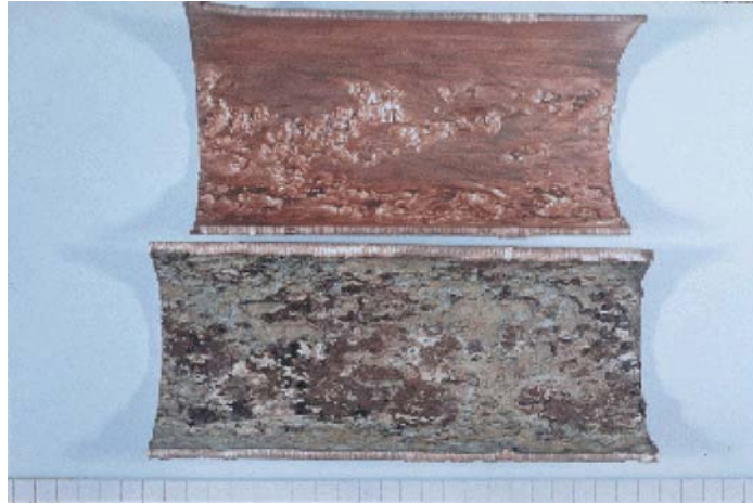
Figure 4-8 Horizontally cut tube ID, tube inlet erosion
