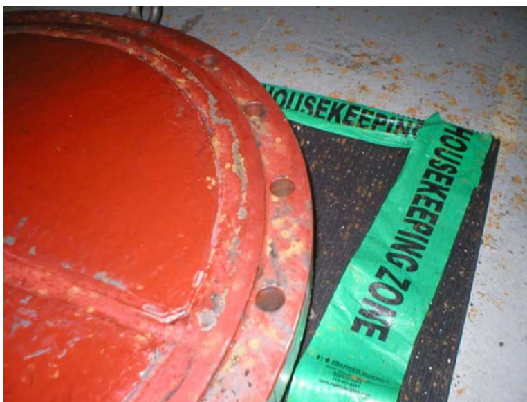
Figure 7-7 Coating failure due to routine and repeated access
