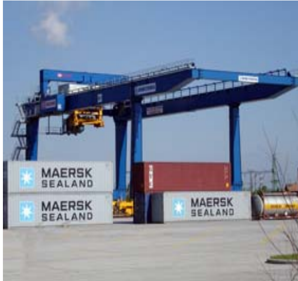
Figure 3-4 A KoneCranes Rail Mounted Gantry Crane
