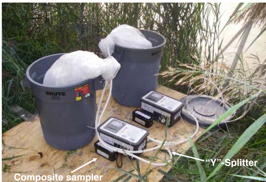
Figure 3-4 Clean Setup for Surface Water Composite Sampling
