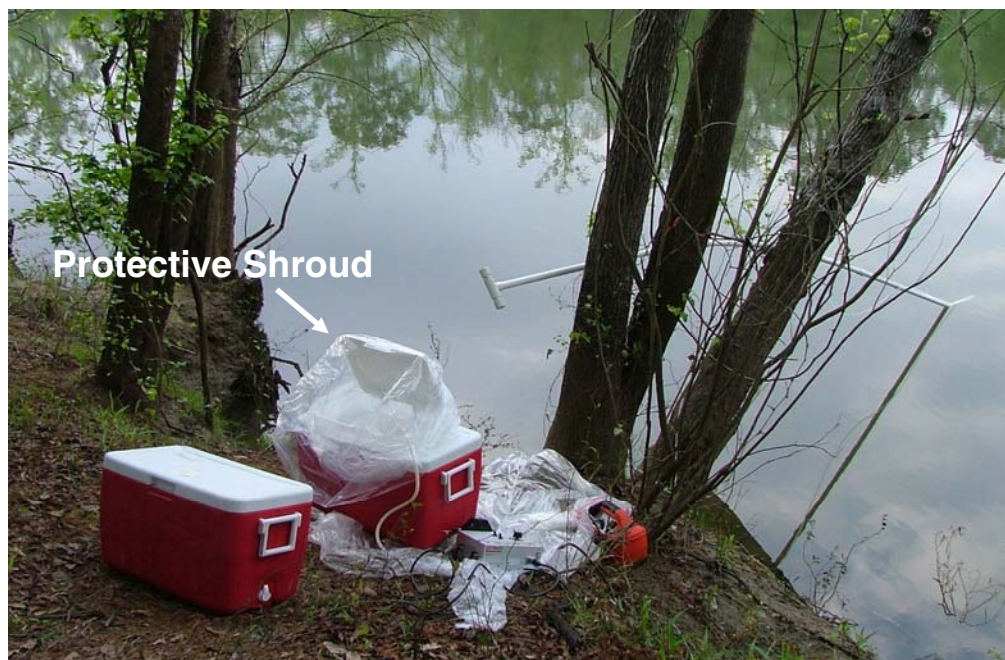
Figure 3-3 Clean Setup for Surface Water Grab Sampling
