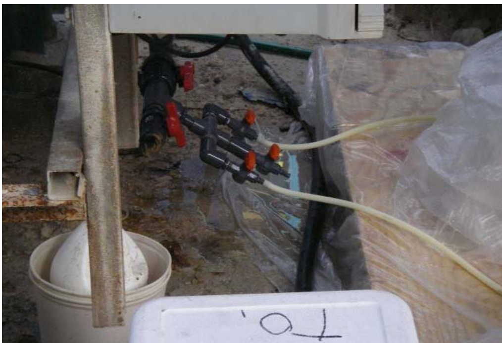
Figure 3-2 Using a Splitter to Collect Replicate Samples
