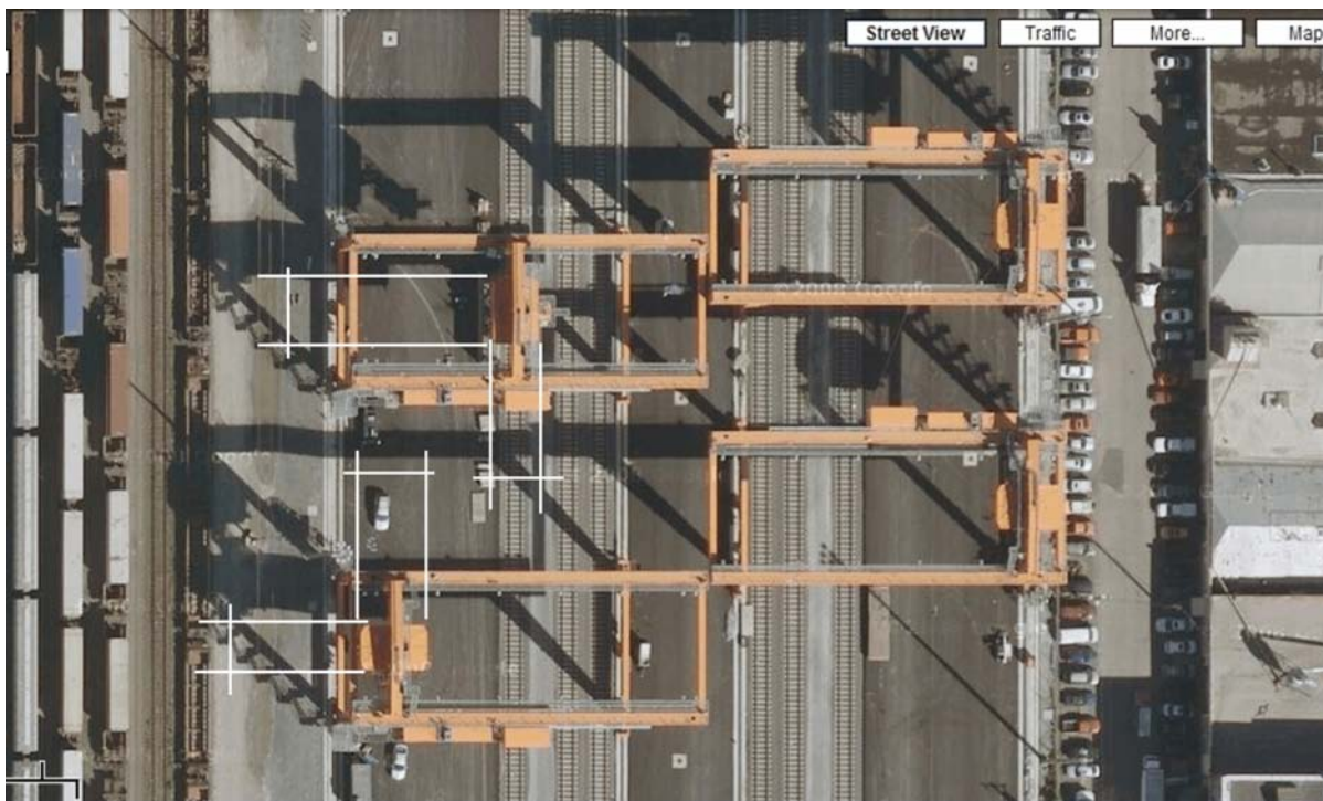
Figure 3-3 Google Earth view of BNSF North SIG Yard RMGs – 90° Rotation Capability of Lifting Carriage
